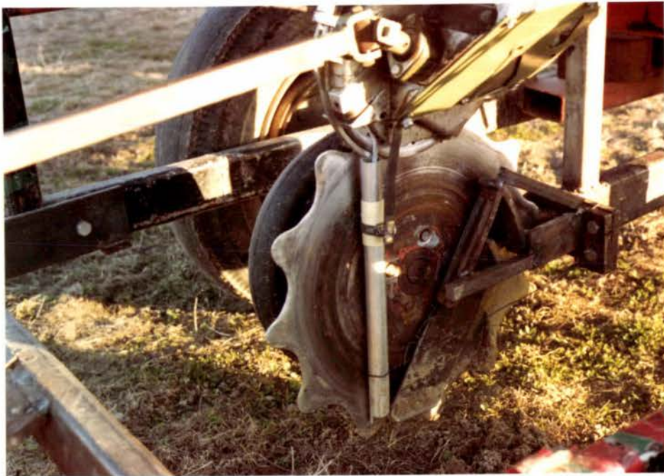
Figure 16: Modified seeder/tube transfer/direct drilling coulter unit operating in a sprayed pasture plot.
