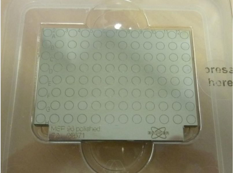
Figure 7. The laboratory bench Microflex LT MALDI-TOF MS set-up (A) and the target plate (B) used for placing samples for analysis.
