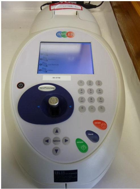
Figure 8. The Implen NanoPhotometer® P300 used to quantify DNA of the 7 isolates sequenced using 16S rDNA.
