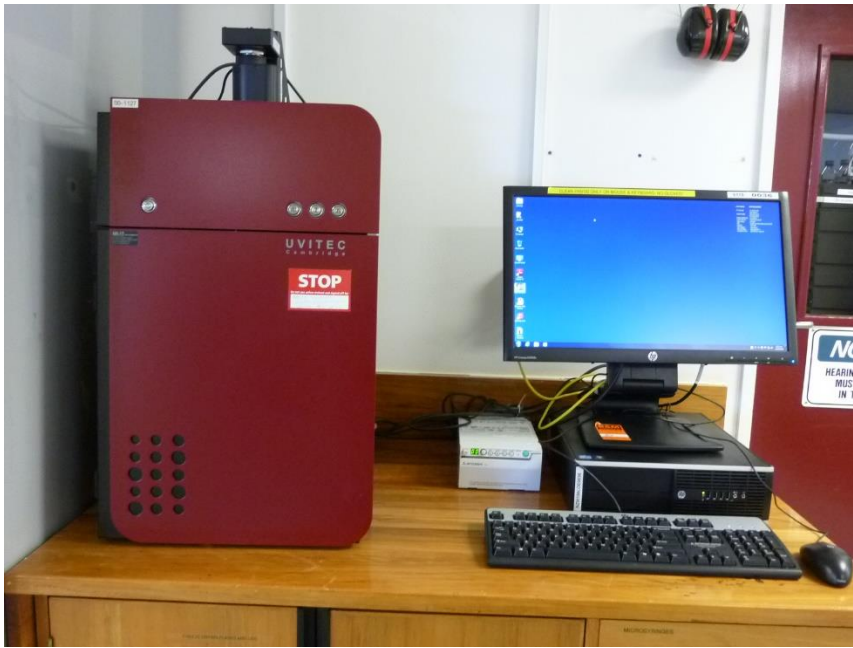
Figure 12. The UVitec Essential V2 used to photograph the gels generated using both the E-Gel system for the SE PCR results and the traditional method for the multiplex PCR results.
