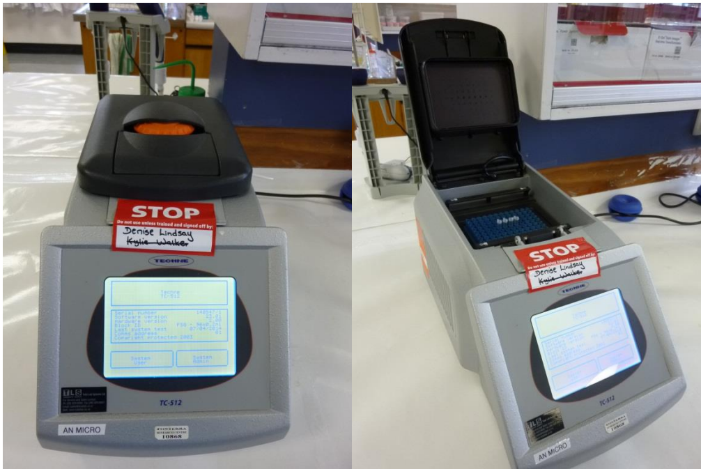
Figure 10. The Techne TC-512 thermal cycler used to generate PCR products for SE PCR, multiplex PCR and 16S rDNA sequencing.
