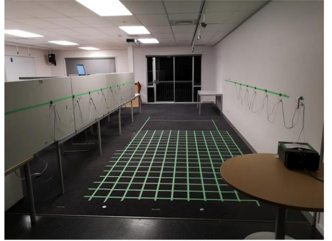
Fig. 5. Experimental setup showing the wall mounted light-sensors and the test space.
