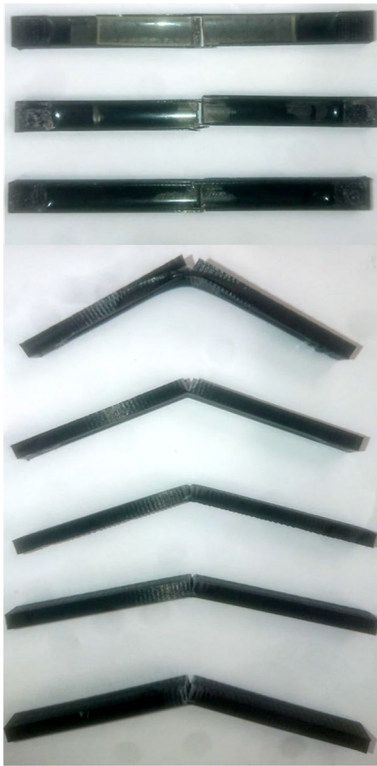
Fig. 15 ABS/epoxy HDM composite samples after flexure testing. Note all are broken with minimum
