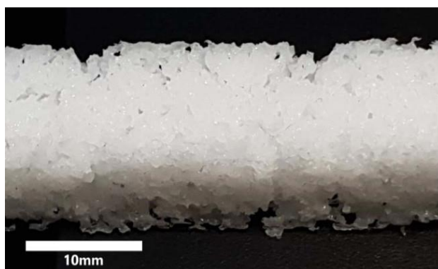
Fig. 6. Close-up image showing a strip of the conductive gel / silicone composite sensor after the gel was dissolved away from the silicone body.
