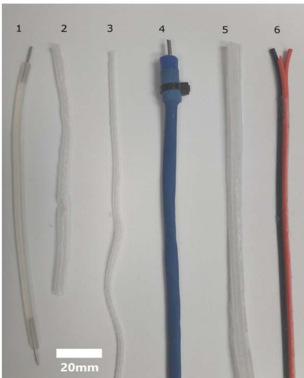
Fig. 2. A selection of trialled sensor materials: (1) commercially available silicone tubing; (2) a thin-walled tube made of silicone; (3) coiled nylon line coated with silicone; (4) a rubber balloon; (5) three tubes sealed together in a triangular shape; (6) a triangular shape made from three silicone-insulated electrical wire sheaths.
