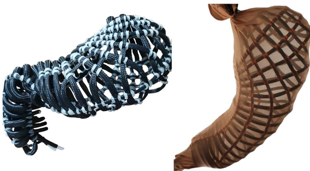
Fig. 29: Examples of interconnected expandable braid artificial muscles forming a 'morphing' stomach shape.
