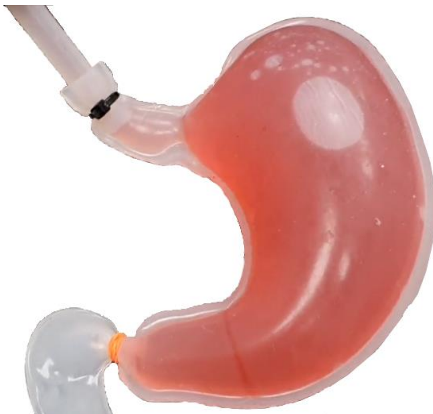
Fig. 15: Transparent inflatable stomach shape made from 100% silicone rubber and filled with coloured water.
