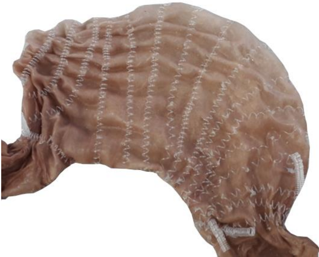
Fig. 32: Direct tying of nylon spring coil unit constrictors onto an artificial membrane surface.
