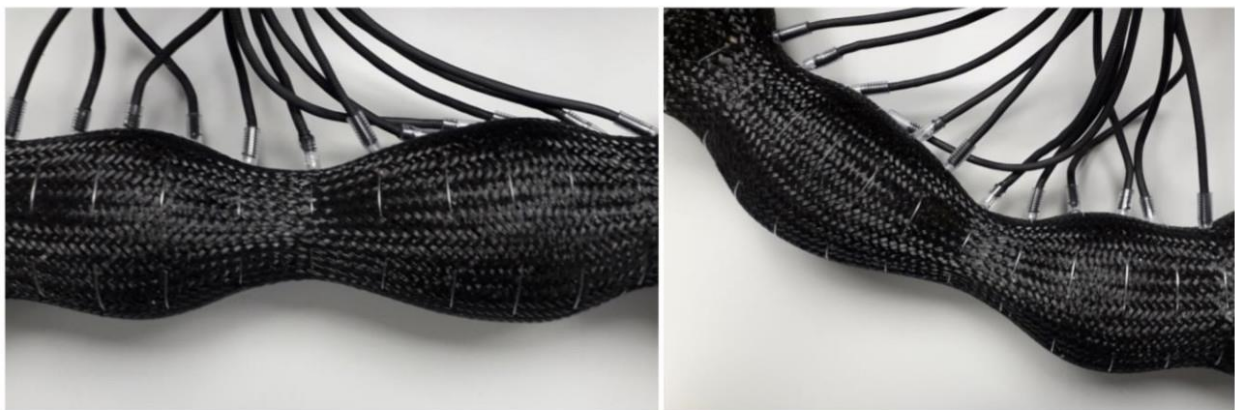
Figure 2: (Left) An example of linear peristaltic waveform deformation of the braided tubing. (Right) A similar deformation pattern is maintained while bending the length of tubing.
