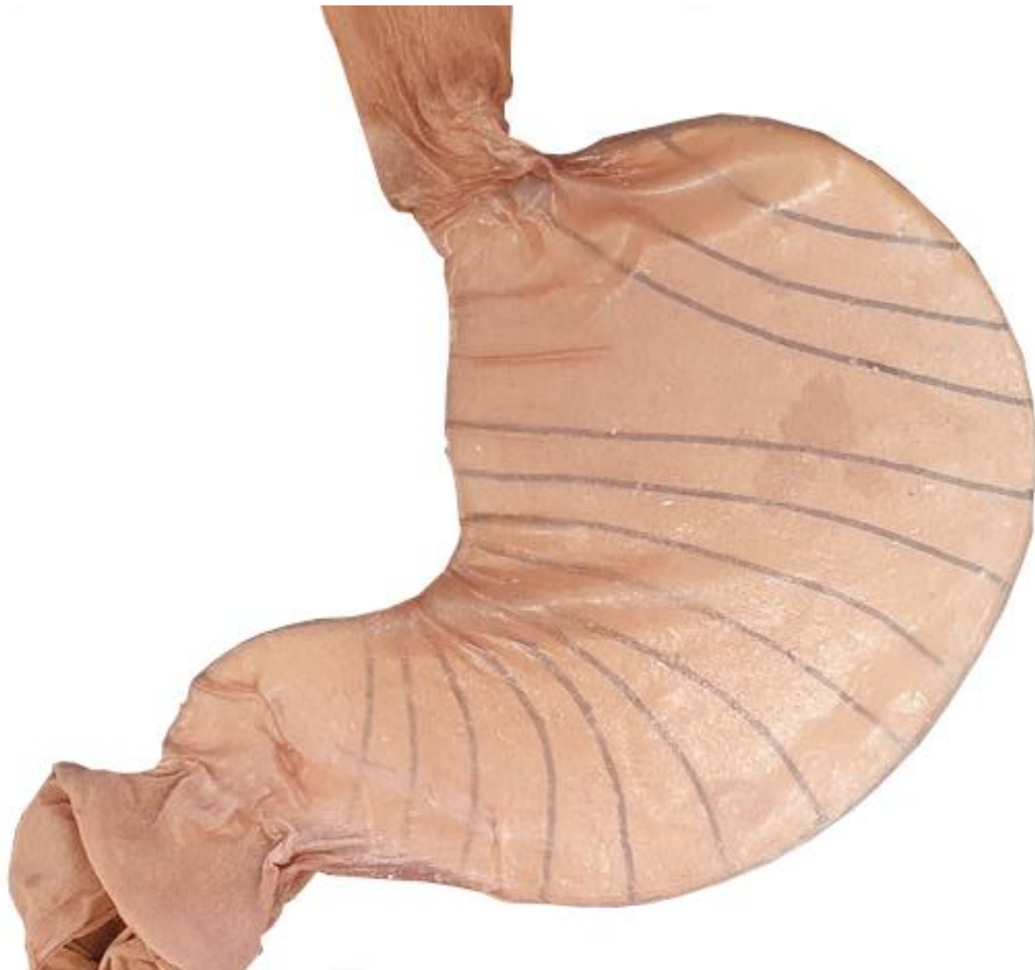
Fig. 9: Composite membrane moulded over the surface of a template stomach form cut from a sheet of MDF.
