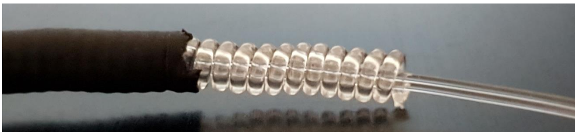
Fig. 35: A nylon coil Bowden cable with a pair of nylon tendons running through it. Part of the outer plastic sheath has been removed to expose the nylon coil.
