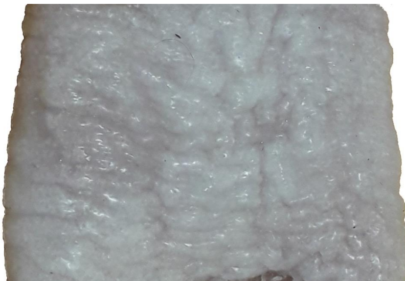
Fig. 21: The appearance of ridges and folding on the surface of the fabricated pre-stressed multi-layer artificial membrane tube prior to turning the tube inside-out.
