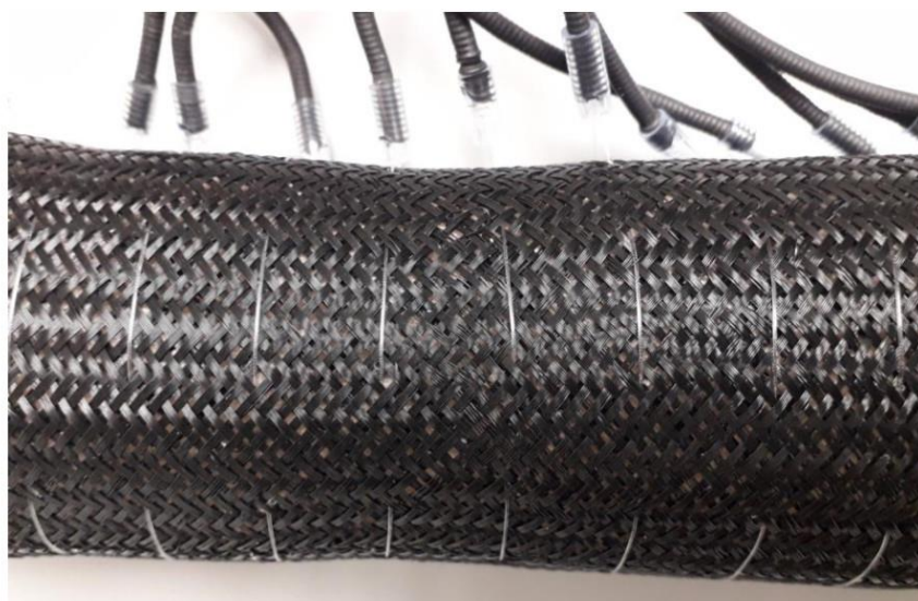
Figure 1: Nylon line constrictors threaded through expandable braided tubing. At the top of the image can be seen Bowden cables through which the constrictor tendons run before connecting to winding spindles.
