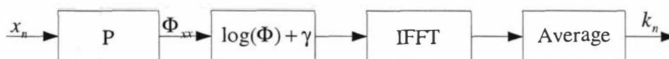
Fig. 4-5 Block diagram for kepstrum processing procedure. (Window: Hanning, \log(\Phi) : log of periodogram, \gamma = Euler constant, 0.577215...)
