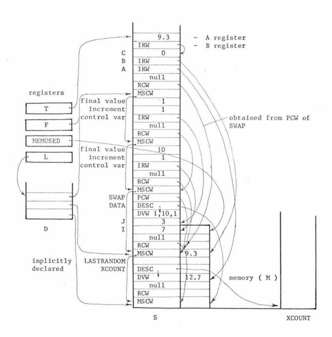
procedure is entered, so the environment will not be the parametered procedure, but its environment. This mechanism is described by Doran [Dora 73]. The word on top of a RCW is used to return the value of the procedure or block and is always present though not always used.
