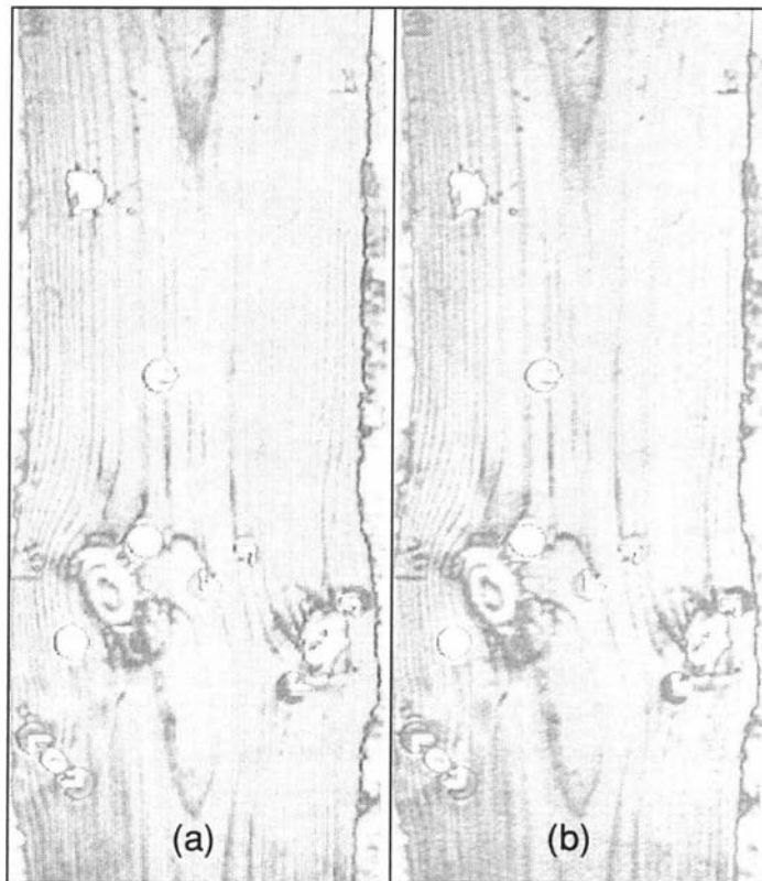
Figure 6.6 Neural network output for experiment 0. Image (a) is the output generated by the network initialized with rules and image (b) is the output generated by the network initialized with random numbers.
