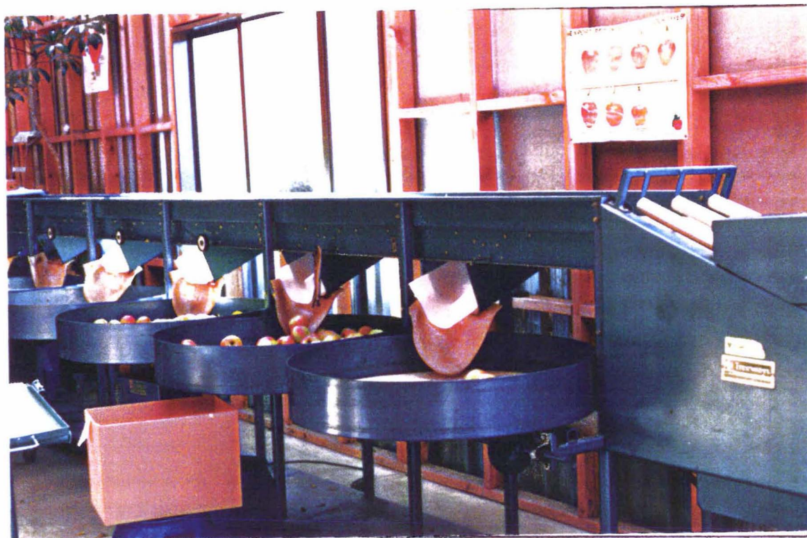
Figure 3.1 Treeways two lane mechanical grading machine used for studying bruise damage
