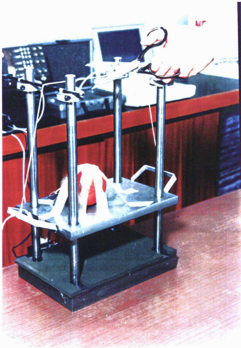
Figure 4.7 Experimental device to calibrate Instrumented Sphere
