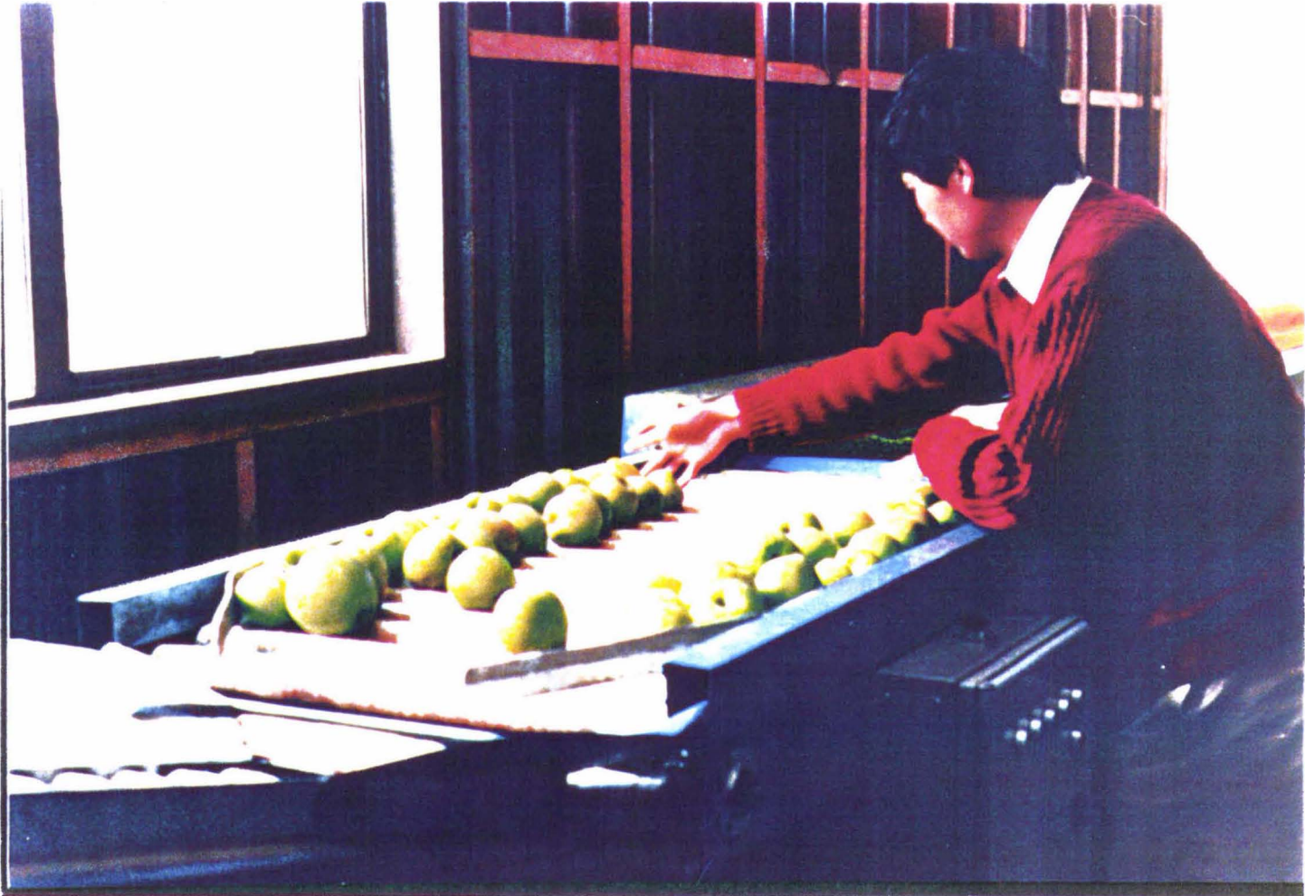
Figure 3.2 Fruit were placed onto sorting table of the grader
