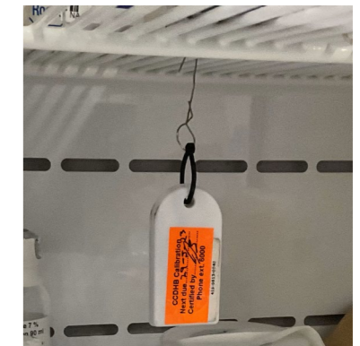
Figure 48. Artefact 02 – Data Logger Suspended by Wire
