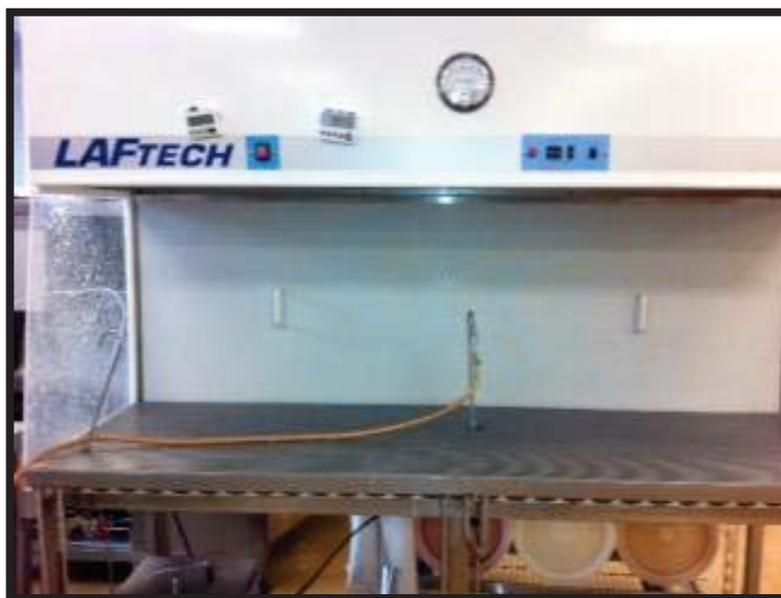
**Figure 3.3 Laminar flow cabinet (Laftech, Victoria, Australia) and filler.**
