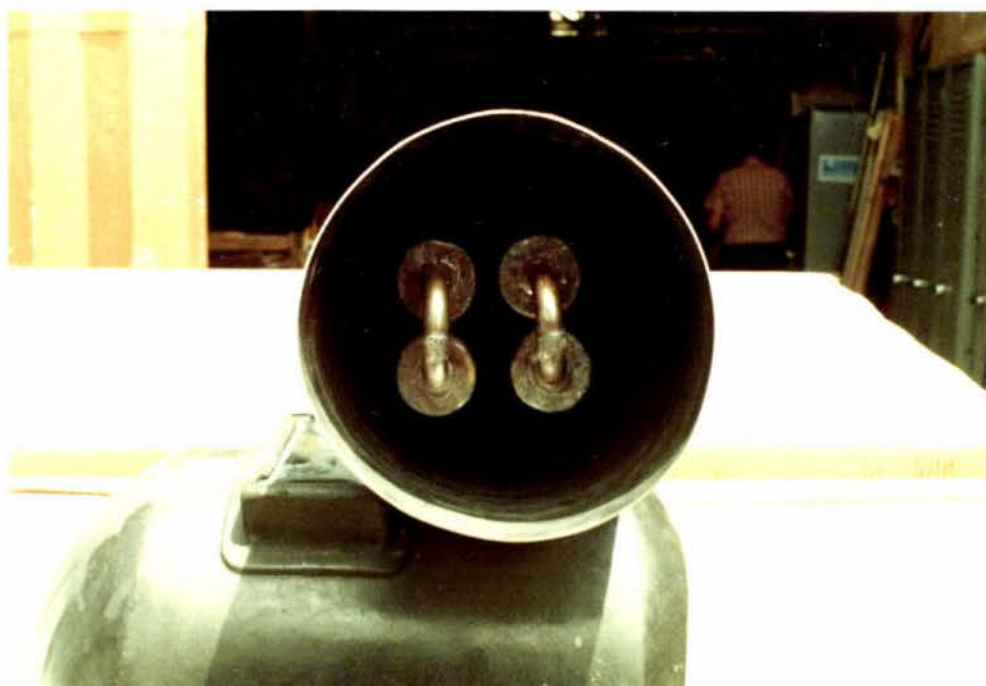
FIGURE 5:7 Plate showing heat exchanger end connection
