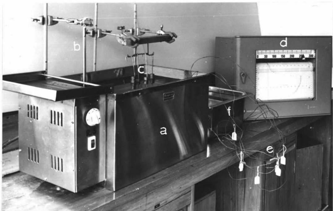
FIG.16. COMPLETE SET UP FOR STERILISATION ON A SMALL SCALE: (a) CONSTANT TEMPERATURE GLYCEROL BATH; (b) THERMOMETER; (c) BRASS TEST TUBE HOLDERS; (d) HONEYWELL TEMPERATURE RECORDER; (e) THERMOCOUPLE LEADS; (f) COOLING BATH.
