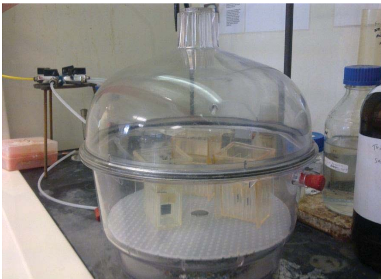
Figure 6.16: Drying process under nitrogen flow
