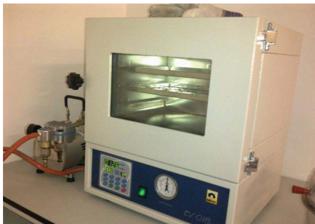
Figure 6.17: Vacuum oven at 120° C for 2 hours
