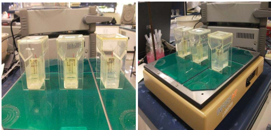
Figure 5.15: 24 hours incubation of sensor in PmB with slow shaker of 125 rpm; FR4 sensors
