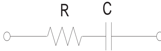
Figure 3.11: A simple series RC equivalent circuit
