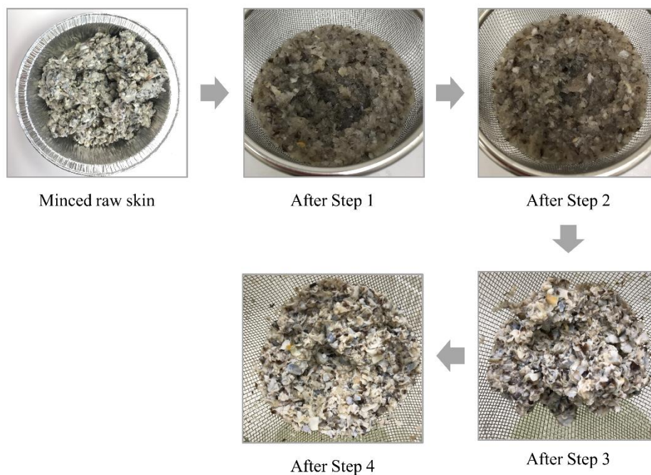
Figure 6.9 Photographs of the fish skin after steps 1-4 of procedure A. Step 1: 0.3 M NaOH wash at 1:10 (m/v) ratio for 90 min; Step 2: 0.3 M NaOH wash at 1:10 (m/v) ratio for 90 min; Step 3: Neutralise with 0.1 M HCl; Step 4: Water wash at 1:10 (m/v) ratio for 90 min.
