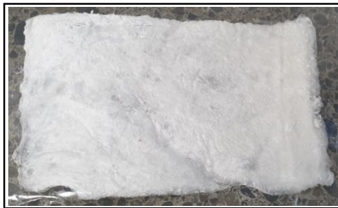
Figure 3.2 Optical photograph of the freeze-dried bovine tendon collagen as viewed by the naked eye.
