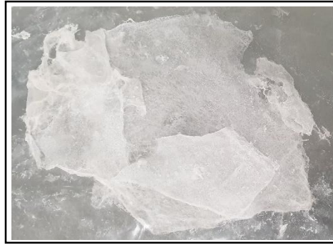
Figure 3.7 Optical photograph of the freeze-dried Tarakihi fish skin collagen from the solution phase.
