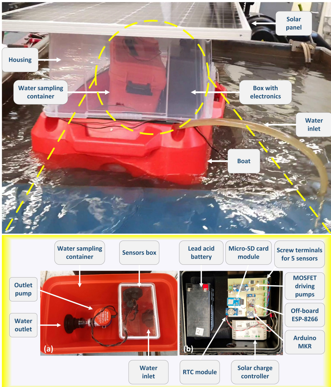
FIGURE 5.6: Initial testing of the system in pool the of water-jet cutter (Top); the system's water sampling container and the electrodes (Bottom)
