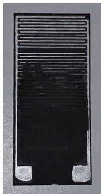
FIGURE 3.5: Warping of 3mm thick acrylic caused by the laser ablation process.
