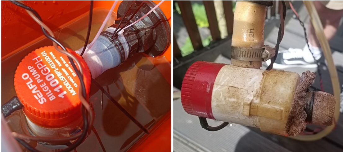
FIGURE 5.10: (left) sediment in water sampling tank, (right) small amount of dirt on inlet pump
