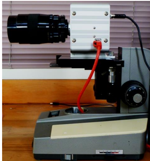
Figure 4-9: High speed camera on an x, y and z moving stage with a macro-lens.
