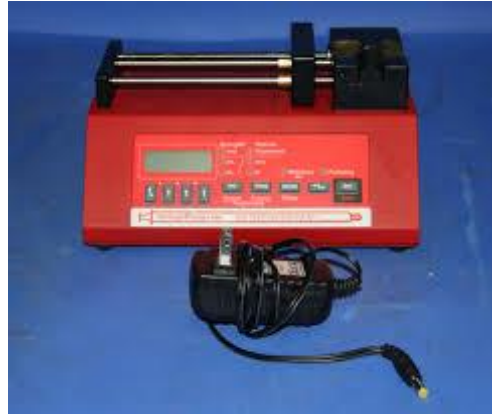
Figure 4-4: Micro-syringe pump to supply bubble liquid and air at the T-junction.
