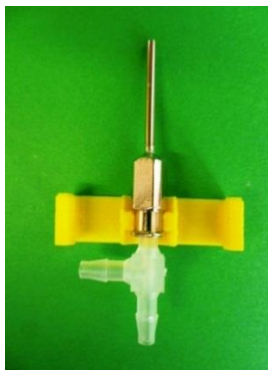
Figure 4-3: Hamilton needle connected with T-junction.
