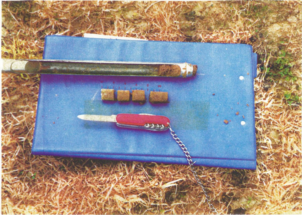
Figure 3.6.6. Sampling method for soil moisture showing core sampler as well as the soil core cut into appropriate sample segments.
