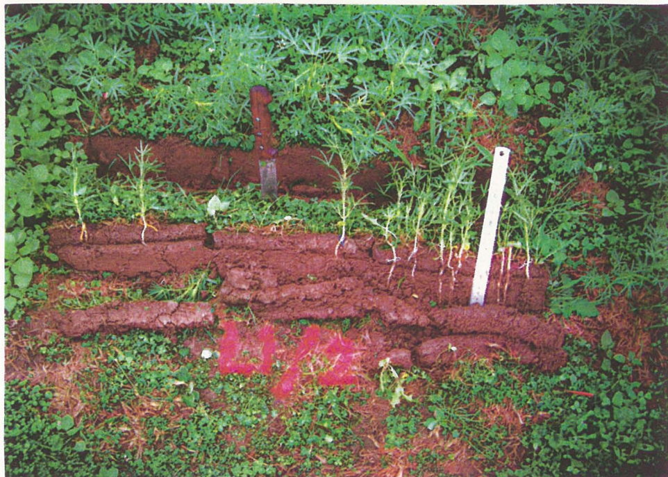
Figure 3.6.4. Measurement of lupin seeding depth showing a clearly defined horizontal ledge in the seeding slot.
