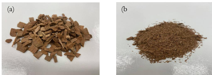
Figure 3-1: (a) Unprocessed kanuka wood chips, (b) kanuka wood chips after being ground and before sieving
