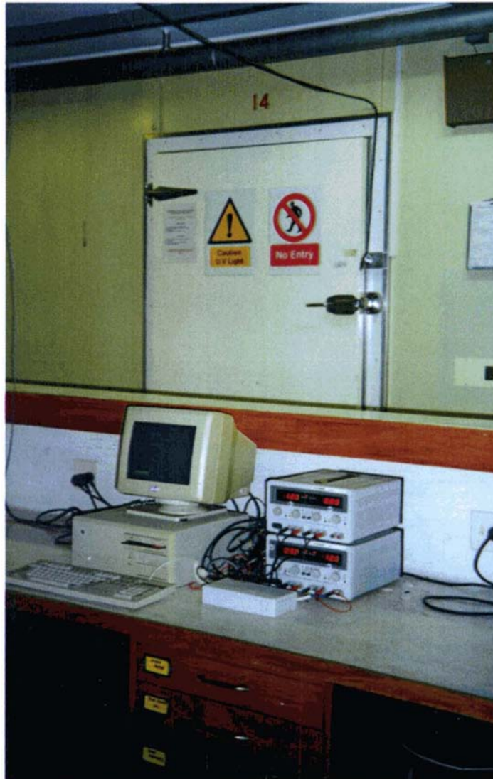
UV-B screening facilities: computer feedback system and walk-in growth chamber
