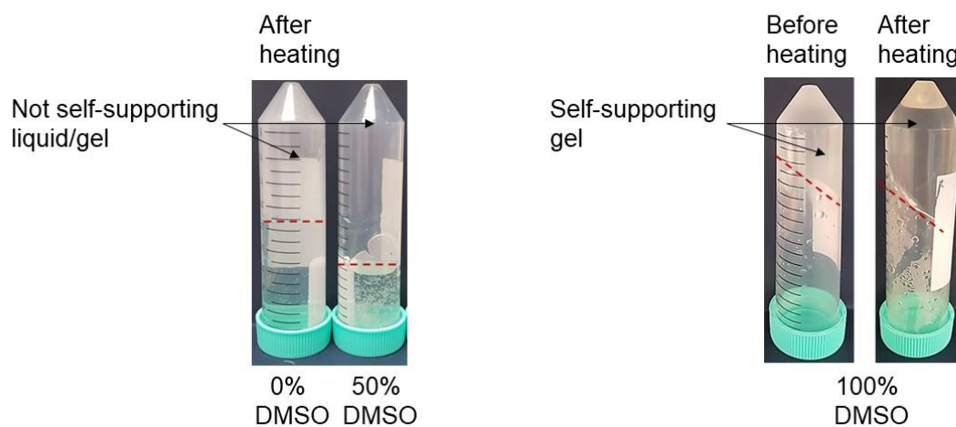
Figure G-2 Effect of DMSO on (A) G' and G'' of 5% w/w 120^\circ\text{C} DWPS before and after shearing at 1000 \text{ s}^{-1} for 5 min. All plotted values are means of two replicates with measurements taken at 20^\circ\text{C} . (B) Photographs showing 5% w/w 120^\circ\text{C} DWPS with 0 and 50% DMSO samples were not self-supporting after heating, and gels containing 100% DMSO were self-supporting before and after heating.
