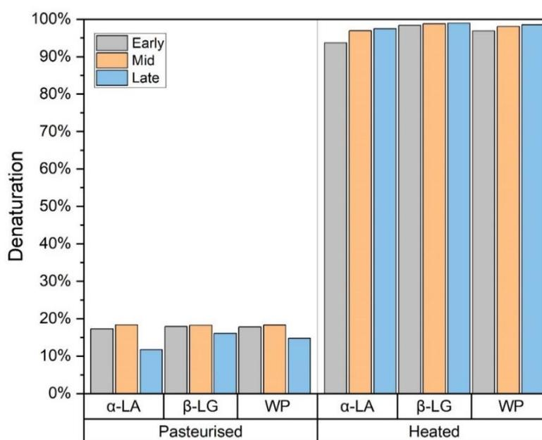
**Figure 5.4** Denaturation level of whey proteins after heat treatment determined by HPLC
