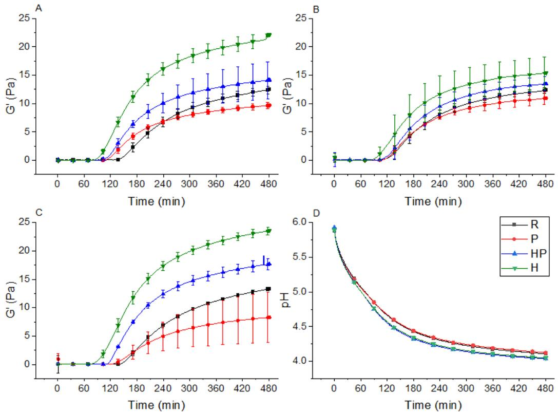
**Figure 4.7** Processing effect on acid gelation properties of spring (A), summer (B), and winter (C) goat milk and pH profile during acidification (D). R - Raw; P - Pasteurised (75°C/15s) without homogenisation; HP - Homogenised and pasteurised (75°C/15s); H - Heated (95°C/5 min) with homogenisation. Error bars indicate the standard deviation of measurements from three different individual experiments.
