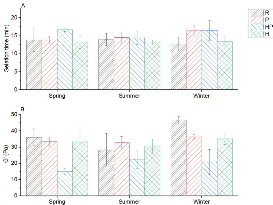
**Figure 4.6** Processing effect on rennet gelation time (A) and final storage modulus (B) of goat milk. R - Raw; P - Pasteurised (75°C/15s) without homogenisation; HP - Homogenised and pasteurised (75°C/15s); H - Heated (95°C/5 min) with homogenisation. Error bars indicate the standard deviation of measurements from three different individual experiments.
