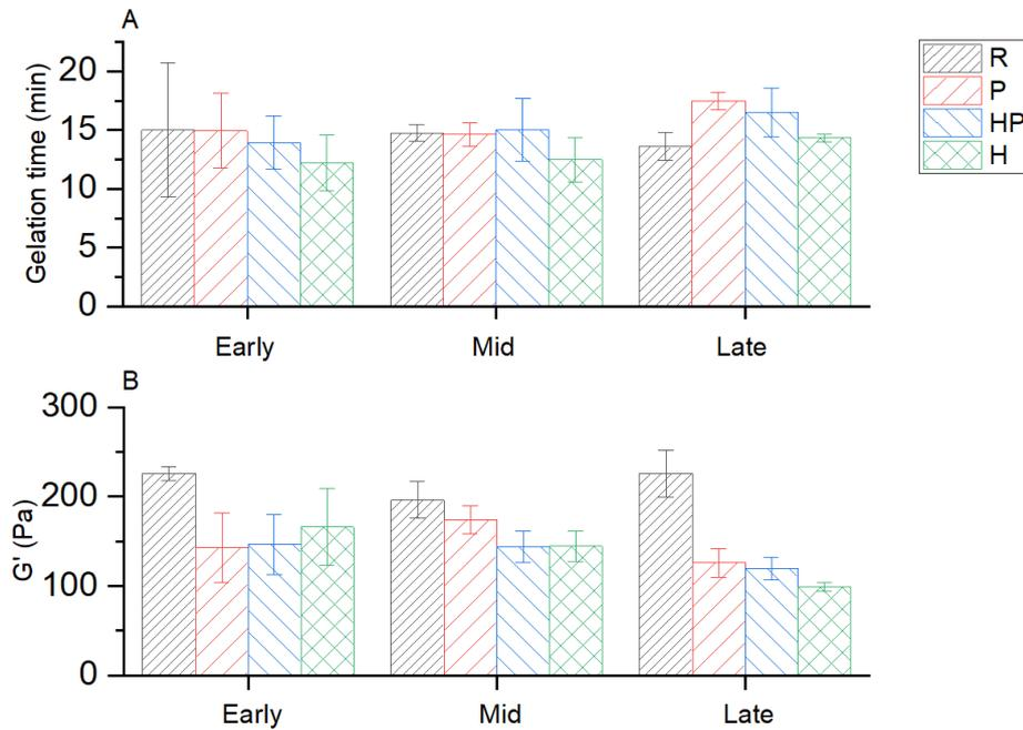
**Figure 5.6** Processing effect on rennet gelation time (A) and final storage modulus (B) of sheep milk; R - Raw; P - Pasteurised (75°C/15s) without homogenisation; HP - Homogenised and pasteurised (75°C/15s); H - Heated (95°C/5 min) with homogenisation. Error bars indicate the standard deviation of measurements from three different individual experiments.
