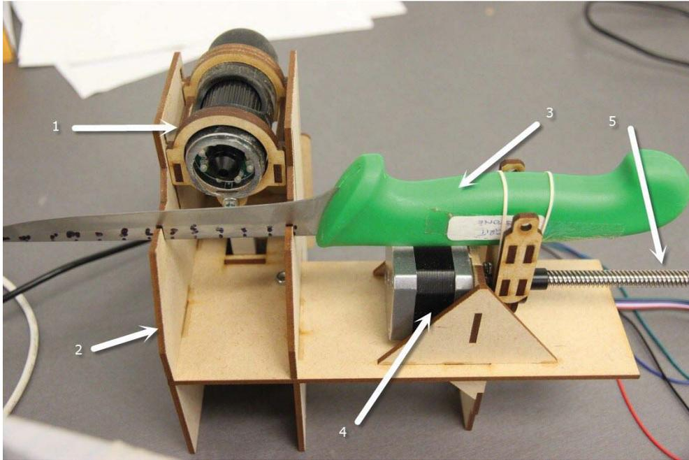
Figure 11: Edge detection in operation. 1 USB microscope, 2 test rig frame, 3 knife, 4 stepper motor, 5 lead screw.
