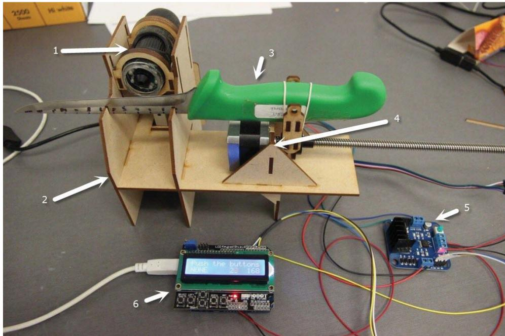
Figure 10: Edge detection test rig with the controller. 1, the USB microscope, 2, the test rig frame, 3, the knife, 4, stepper motor to move the knife, 5, the stepper motor controller and 6, the Arduino controller.
