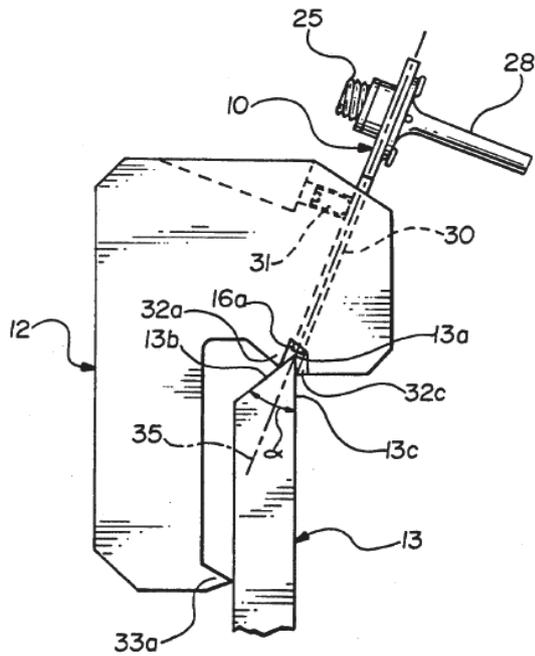
Figure 8: US5196800 (1993) Capacitance sensor probe, 13 - knife blade, 16 - capacitance probe point, 25 - probe body, 12 - sensor mount, 33a - knife guide.
