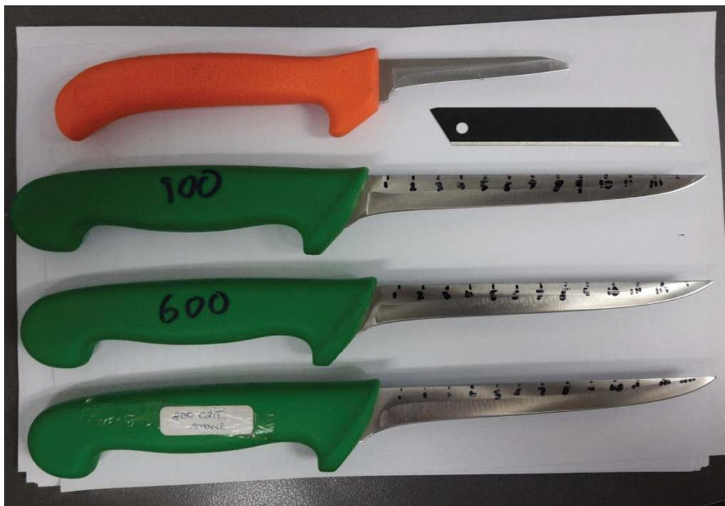
*Figure 9: The knives used in the testing. Top to bottom, orange knife, box cutter razor, 900 grit, 600 grit, and 400 grit.*
