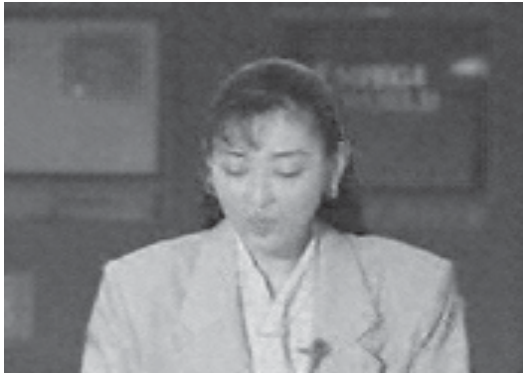
7.16.b: Akiyo Proposed Reconstruction, PSNR= 32.70dB, SSIM Index= 0.89
