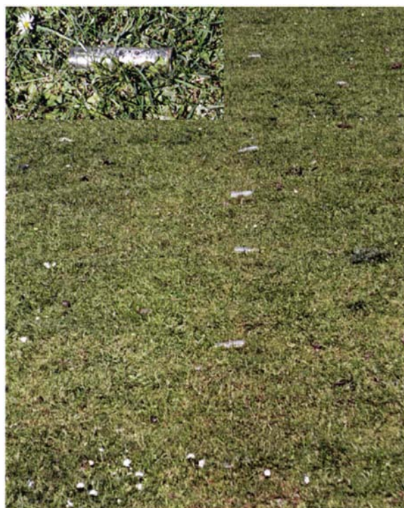
Plate 3.2: Ammonia volatilisation measurement using passive samplers (Carran et al. , 2000).
