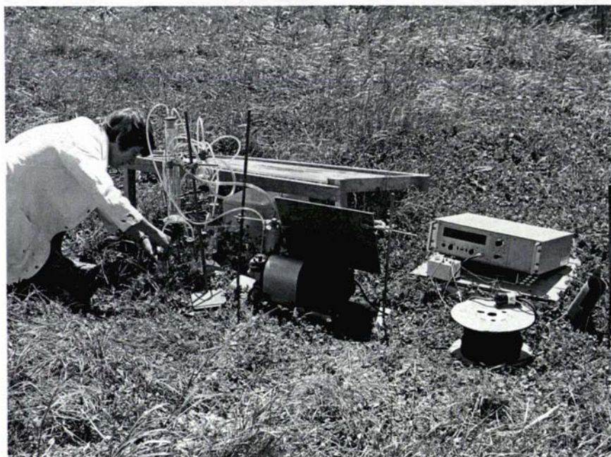
Plate 3.1: Ammonia volatilisation measurement using chamber methods (Ball et al. , 1979; Theobald, 1983).
