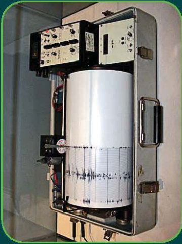
Above: Seismographs measure ground shaking and record it onto a drum. They provide important information which is used to locate, measure and study earthquakes.
