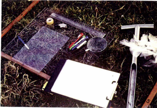
Plate 6.1. Material used to collect data in the field. Note especially the use of a sheet of plain glass and acetate for mapping.
