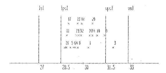
Figure 4.1 Screen layout of Pre-control chart
