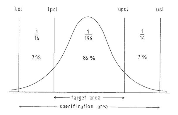
Figure 2.1 The location of Pre-control limits (Traver, 1985)
