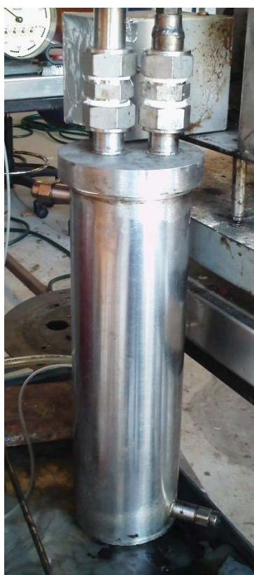
Figure B-3. Condenser for Binder Burner. Designed as a counter current double hull condenser. The height, inner diameter, and hull thickness is 30 cm, 10 cm, and 3 mm respectively.
