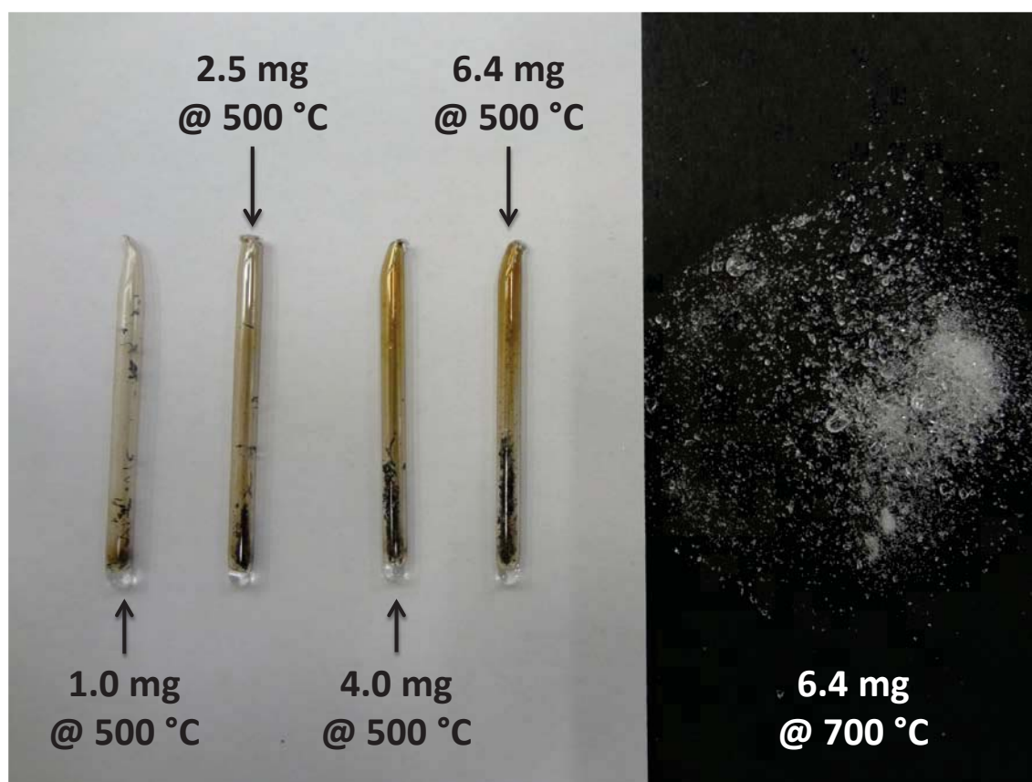
Figure 6-12. Glass capsule pressure test. The weights in the figure refer to the feedstock weight initially sealed in the respective capsule, and the subsequently stated temperature is the set point temperature to which the electric furnace was heated in the respective experiment. The picture on the right depicts the remnants of a broken capsule and the conditions which led to its destruction.
