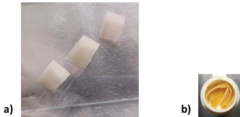
Figure 3-3. Final positioning of cut pine shavings. a) Small strips of radiata pine with a length of approximately 5 to 10 mm and a width/height of \approx 4 mm. b) Positioning of shavings in crucible. The crucible is an Alumina crucible with a diameter of 5 mm and height of 4 mm.
