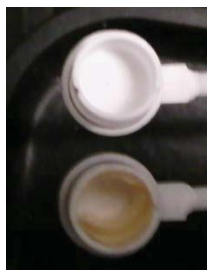
Figure 3-20. Example of placement of slices in “LTGA—EW; slices & cuboids” experiments in Figure 3-19. In this example three slices were placed next to each other having an average thickness of 0.06 mm. The crucible is an Alumina crucible with a diameter of 5 mm and height of 4 mm.
