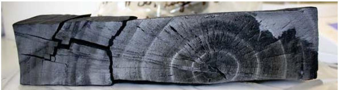
Figure 3-31. Cracks and fractures in a cuboid sample beam with a length of approximately 175 mm and a cross section of 67 x 67 mm pyrolysed to \approx 400 °C. Picture taken from Bashir (2012).
