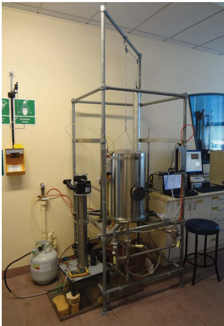
Figure B-1. Binder Burner (Macro-TGA) with peripheral equipment.
