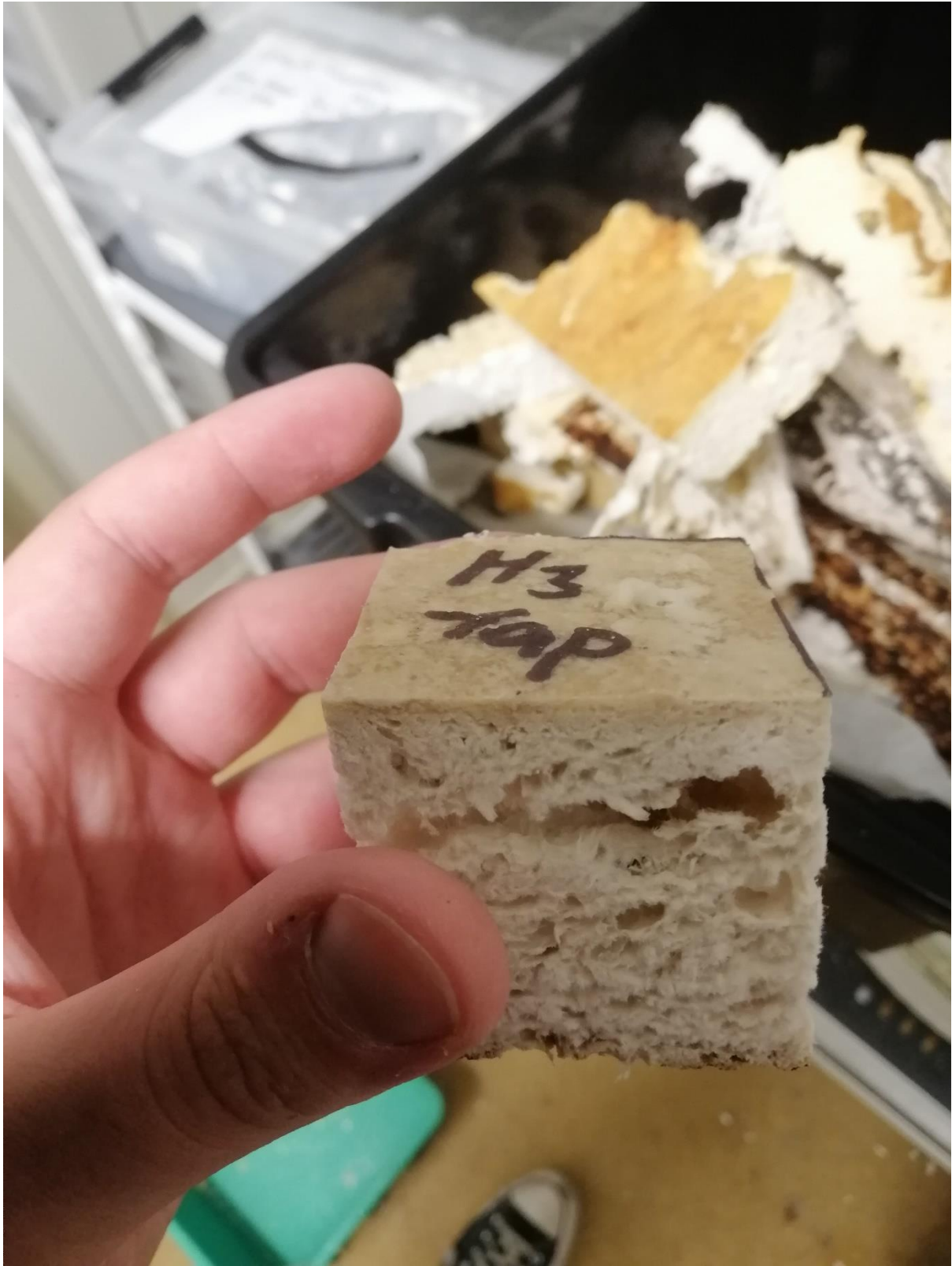
Figure 24: Cross section of tapioca starch panel.
