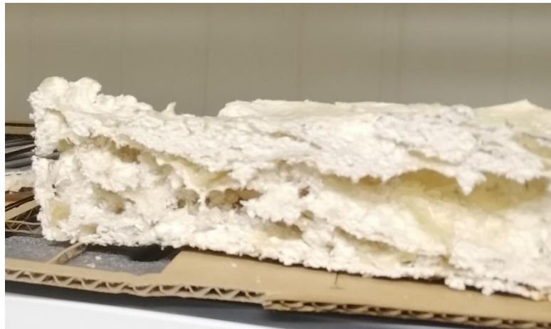
Figure 25: Cross section of the potato starch panel, showing lots of air gaps in its internal structure.
