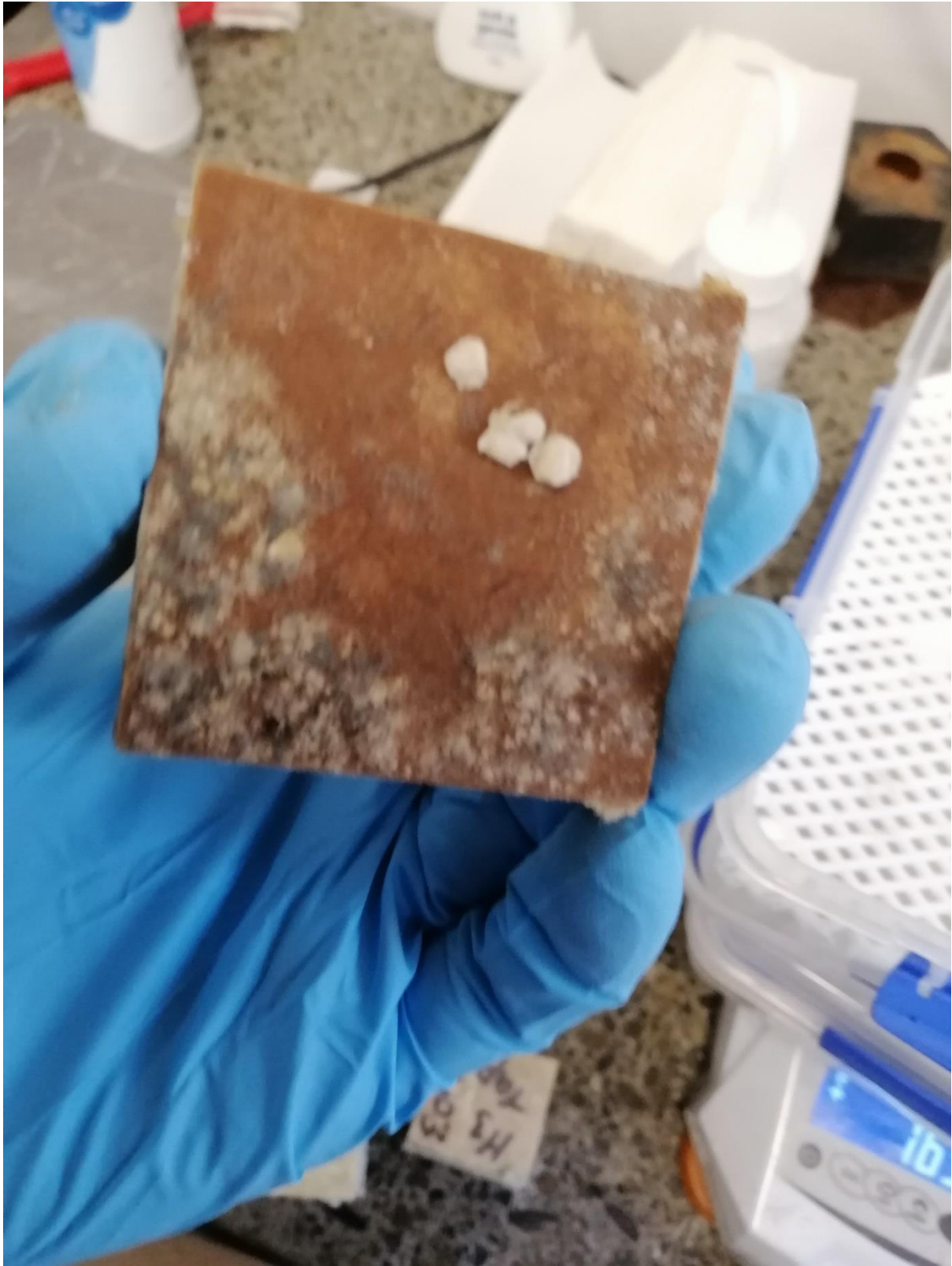
Figure 47: Close up of rear of MDF after exposure to KNO_3
