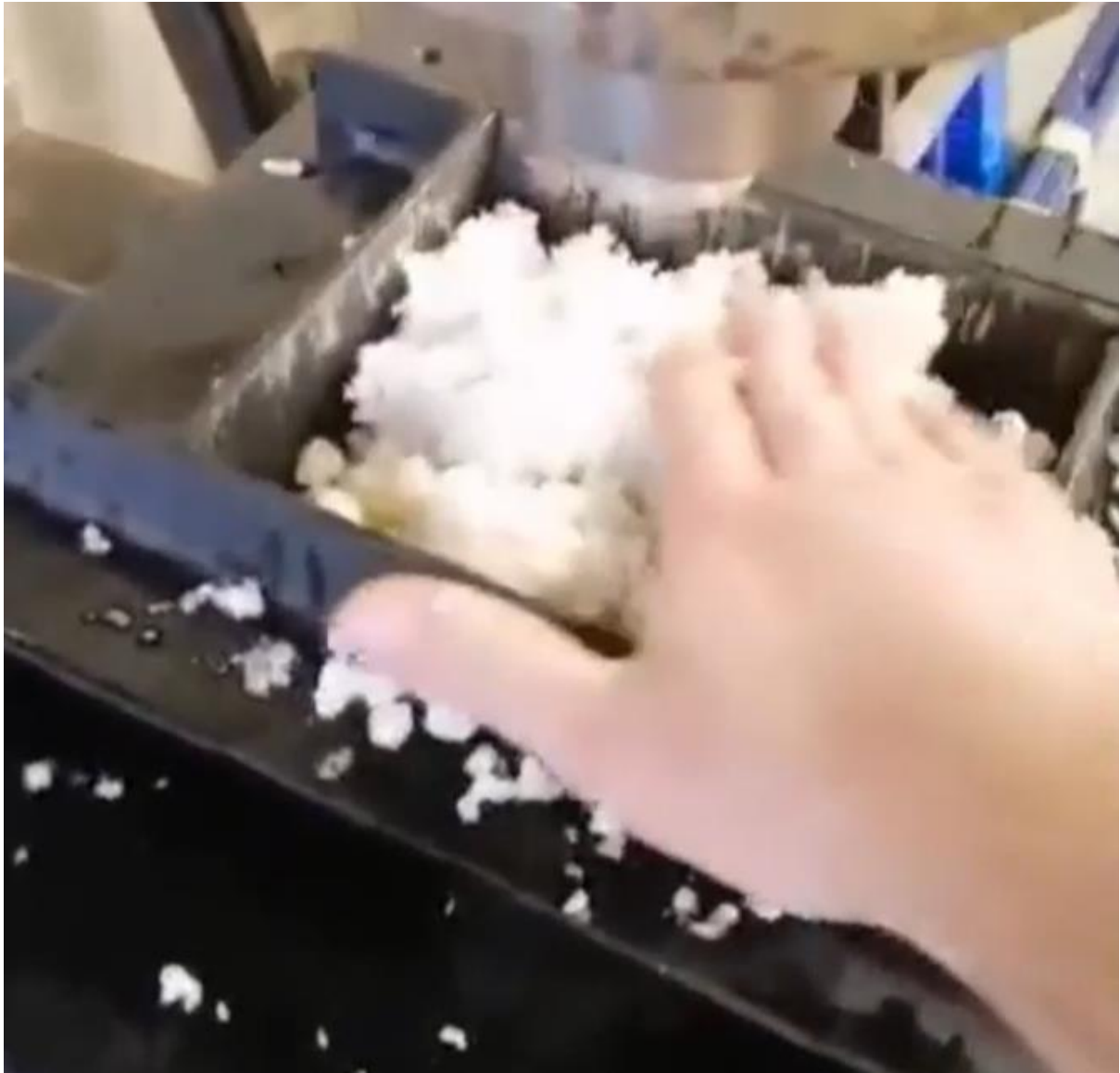
Figure 8: Inserting pulp into small mould manually.
