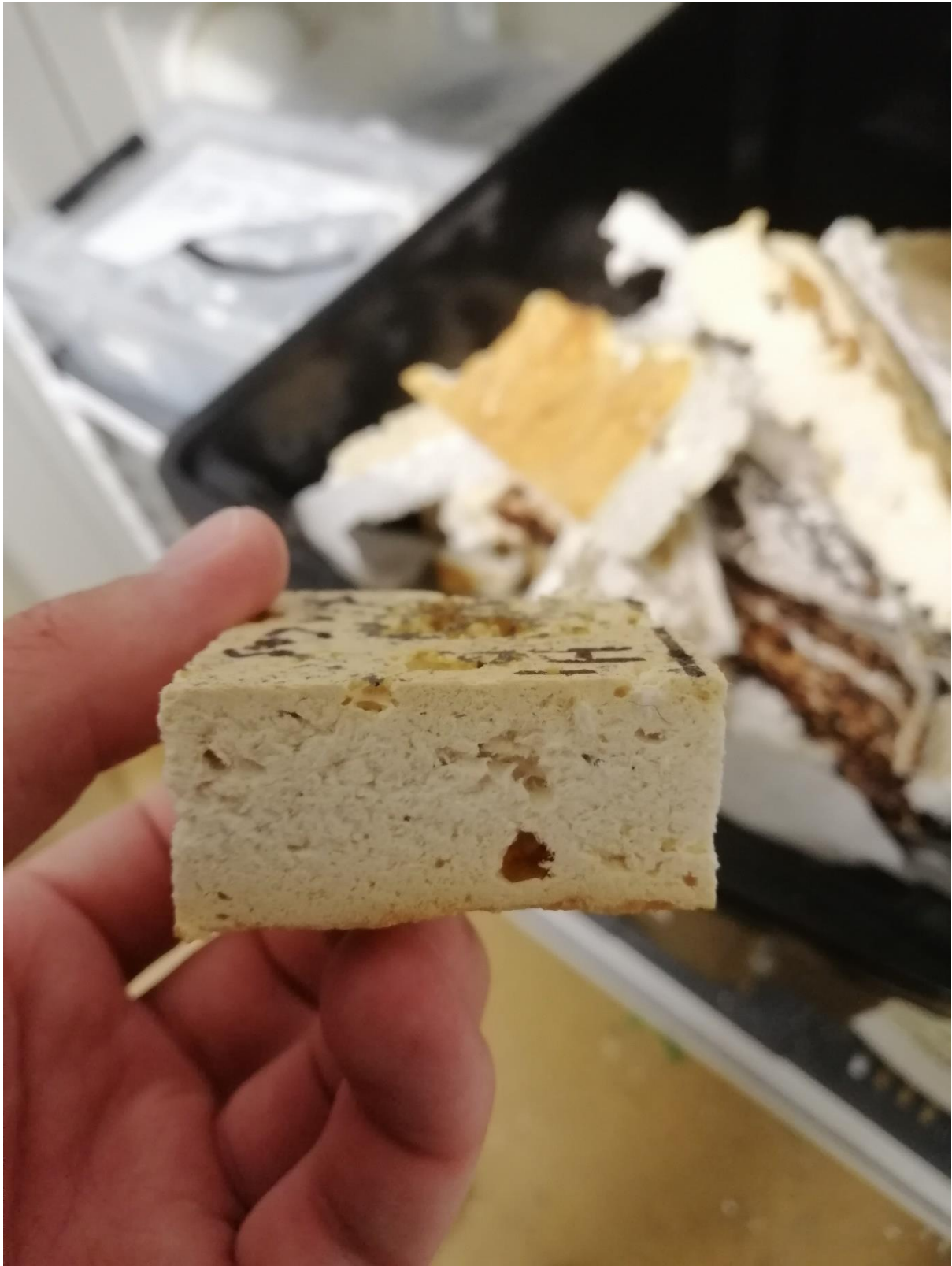
Figure 32: Cross section of casein panel.
