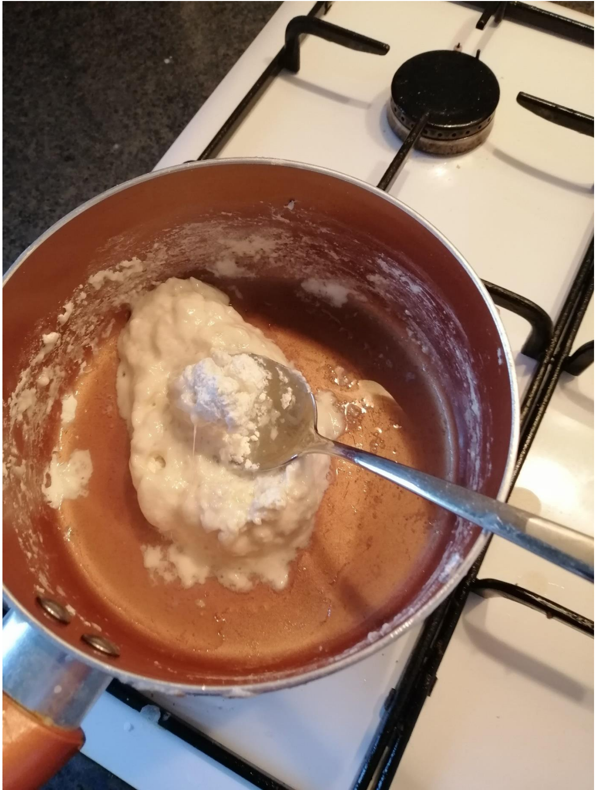
Figure 29: Very sticky casein glue formed that started to harden quickly.
