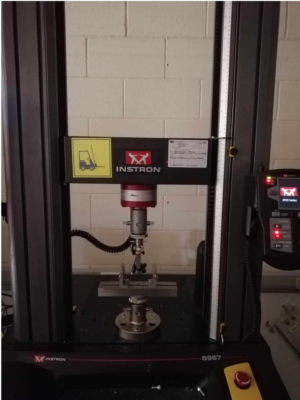
Figure 36: 3-point bending test apparatus
