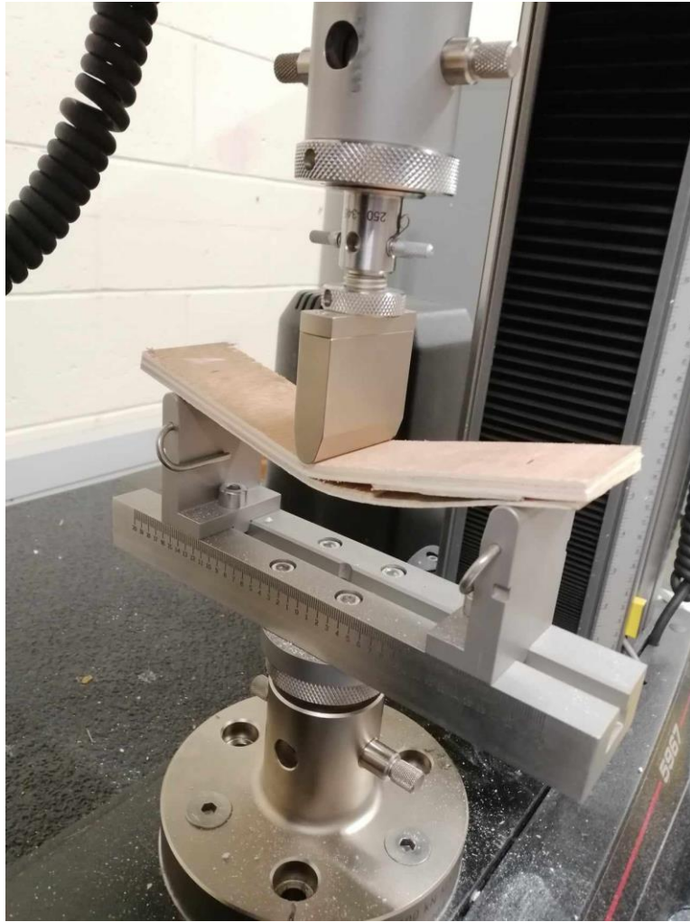
Figure 56: Bending test on plywood sample
