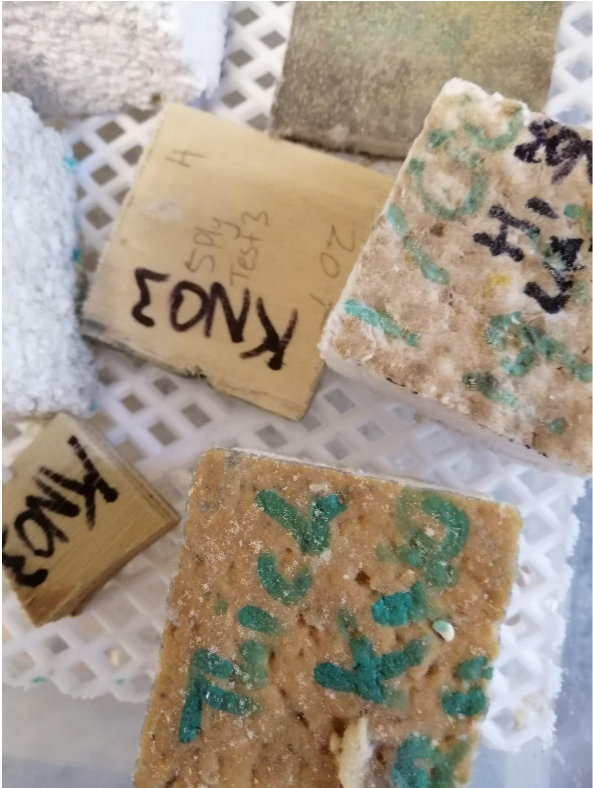
Figure 45: Close up of Casein Panel after exposure to KNO_3
