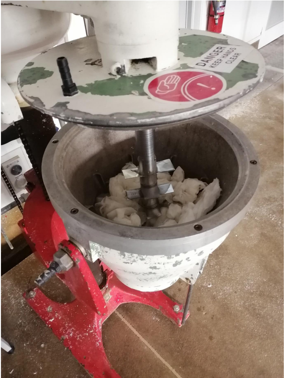
Figure 6: Filled wet disintegrator bucket before pulping.
