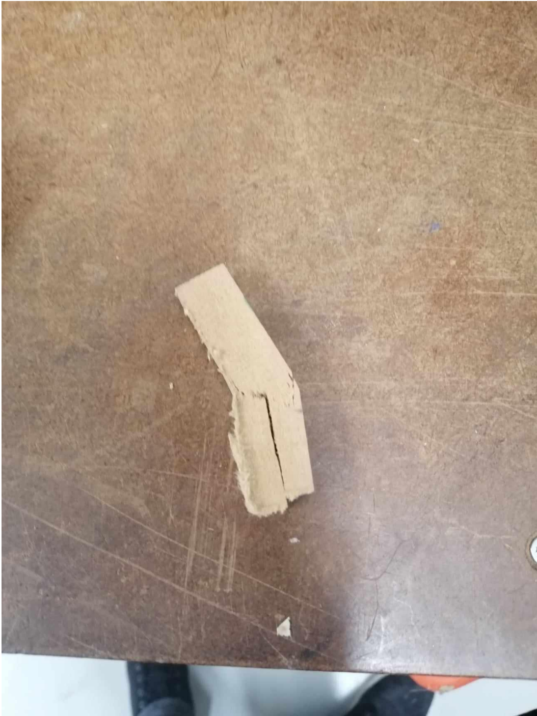
Figure 58: MDF sample failure after impact
