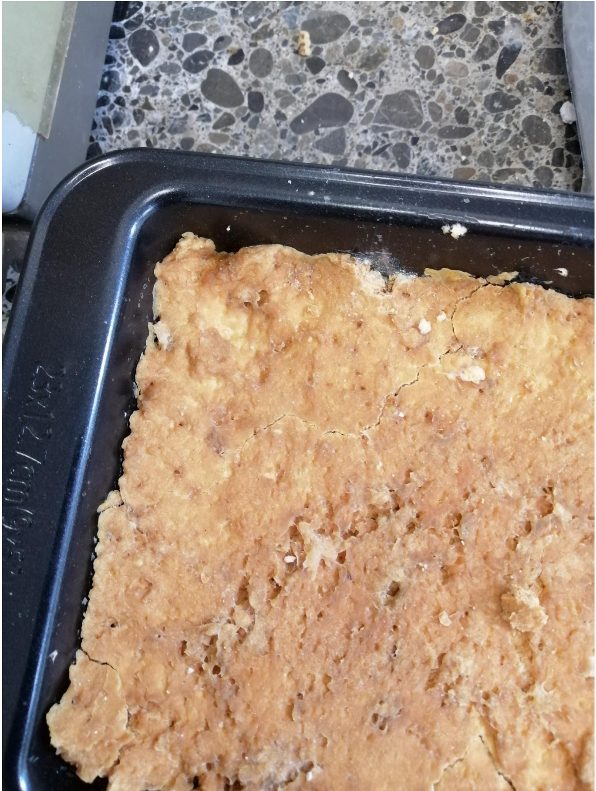
Figure 31: Casein panel in ingot shaped cake tins.
