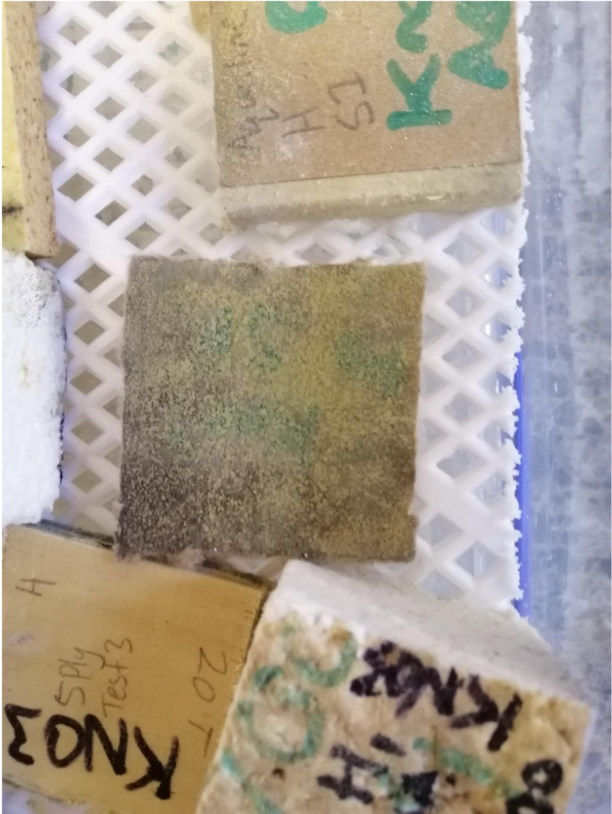
Figure 44: Close up of Sheetrock (GIB) (unreadable panel) after exposure to KNO_3
