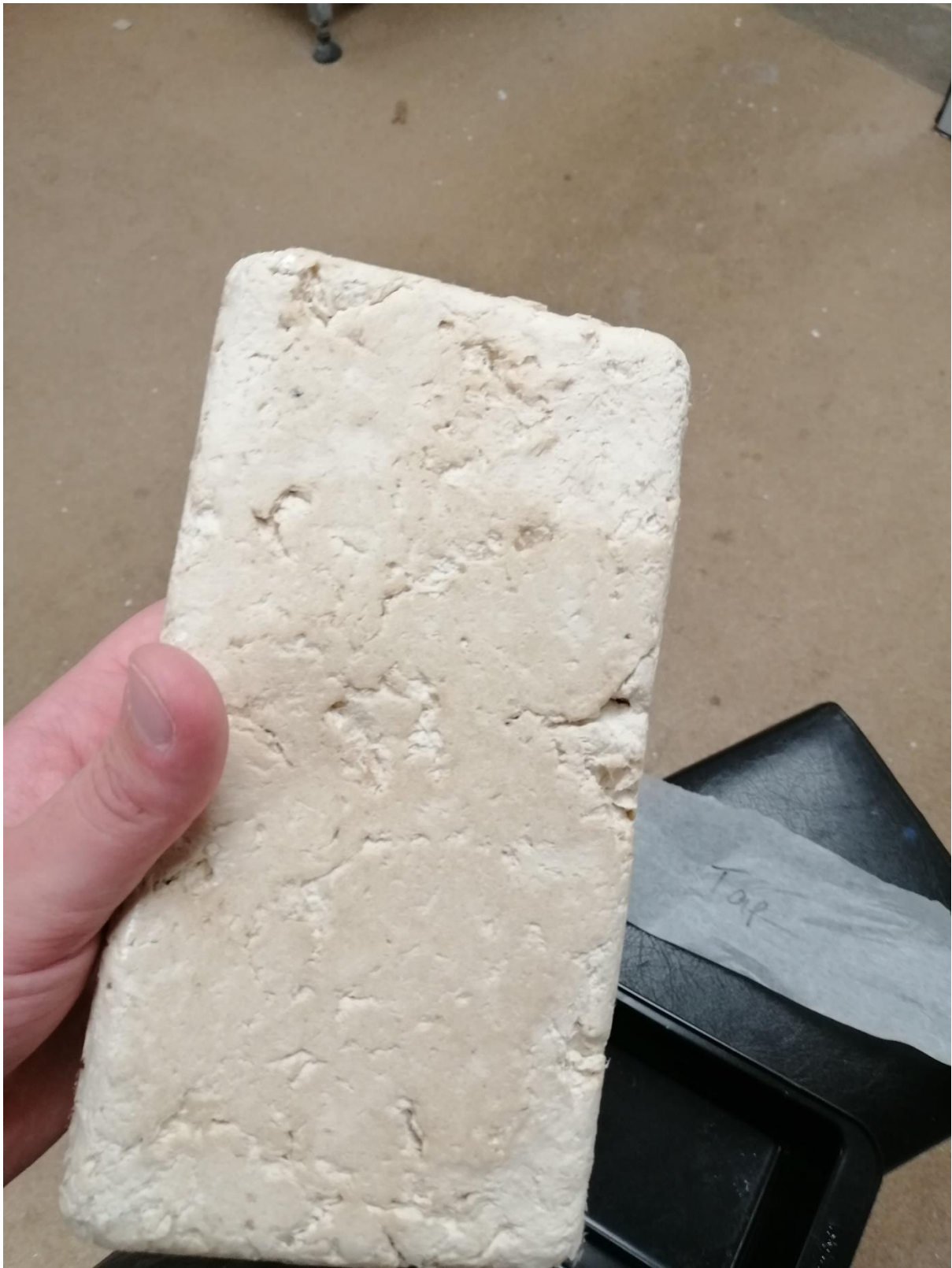
Figure 27: Tapioca panel made from rectangular cake tin.
