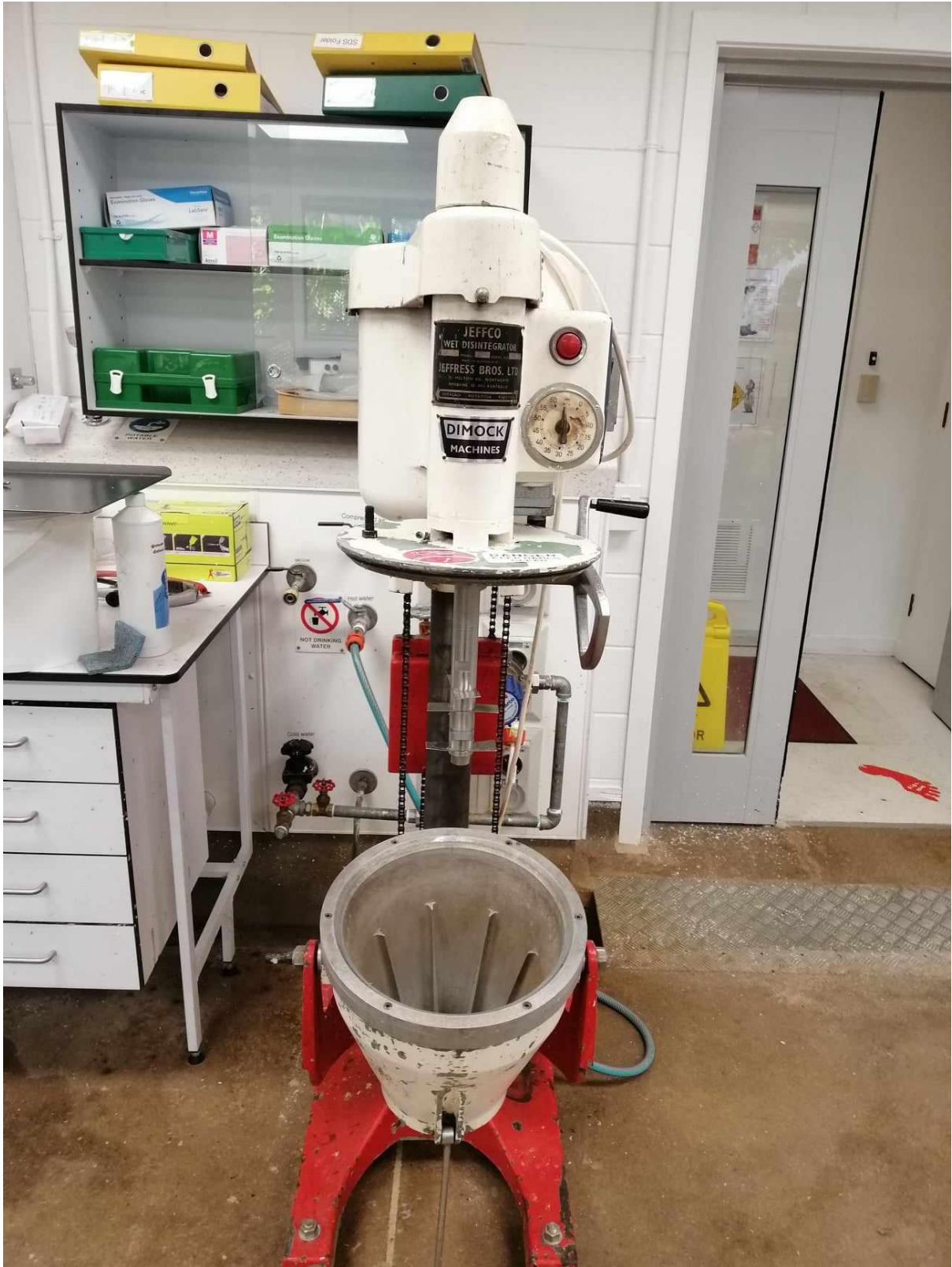
Figure 5: Wet disintegrator (before putting paper towels in)
