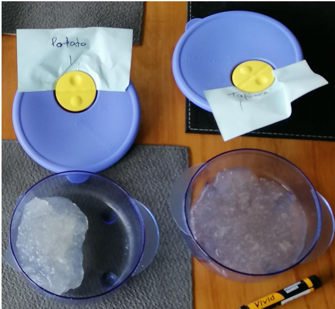
Figure 21: Solidified potato starch (left) and solidified tapioca starch (right).
