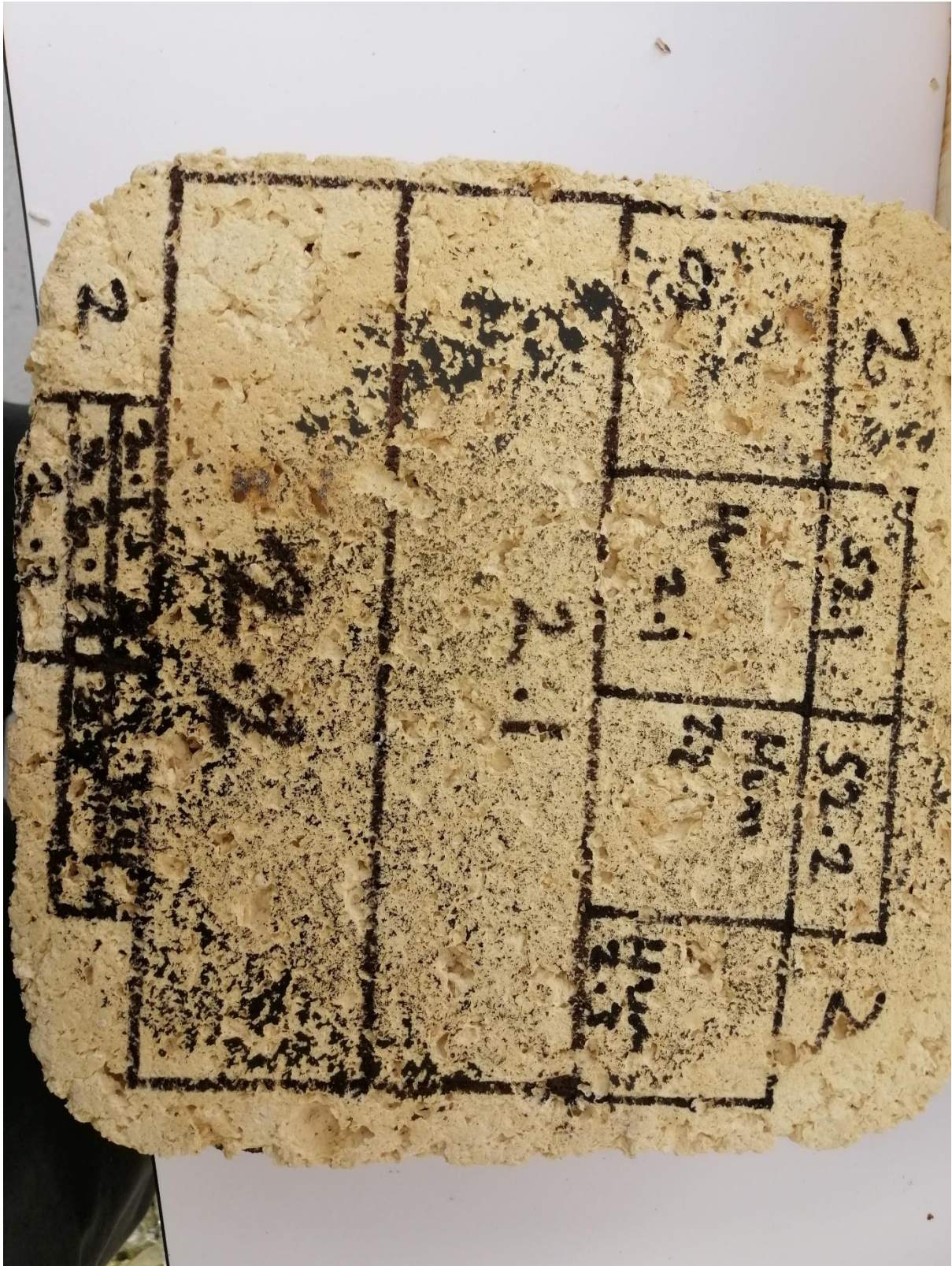
Figure 33: Casein panel made from square cake tins.
