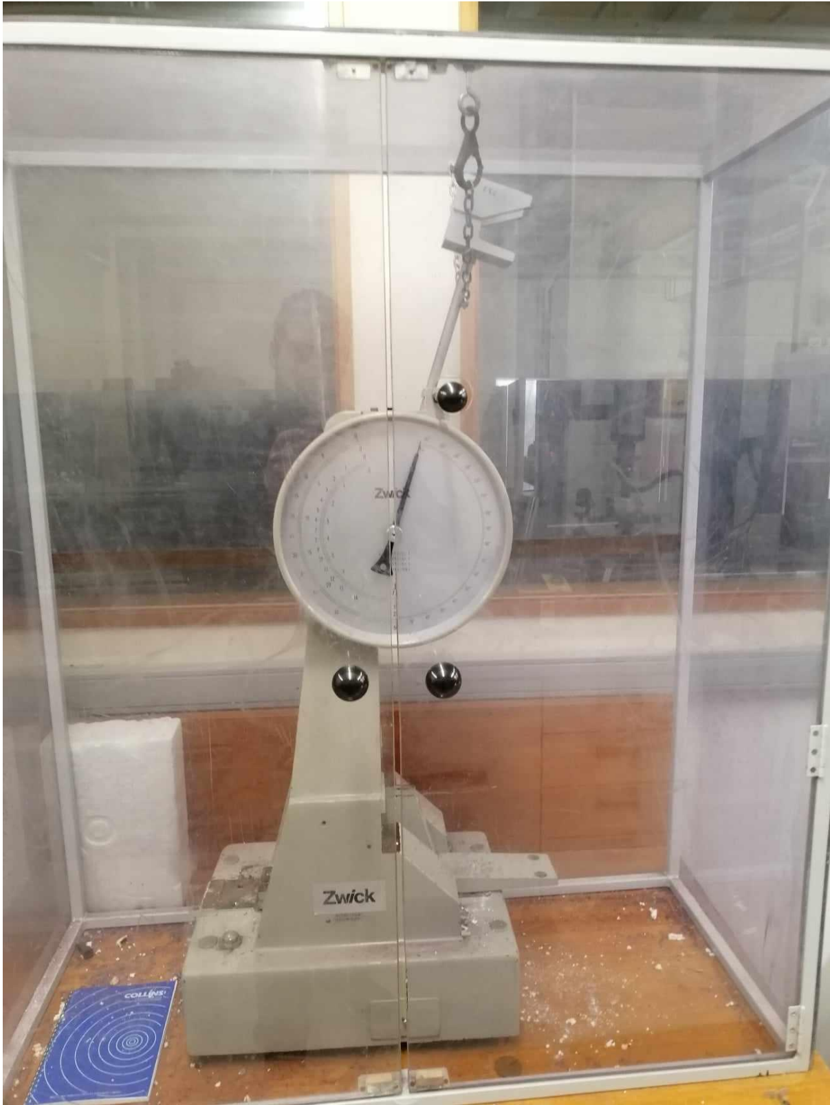
Figure 37: Impact tester used with pendulum arm
