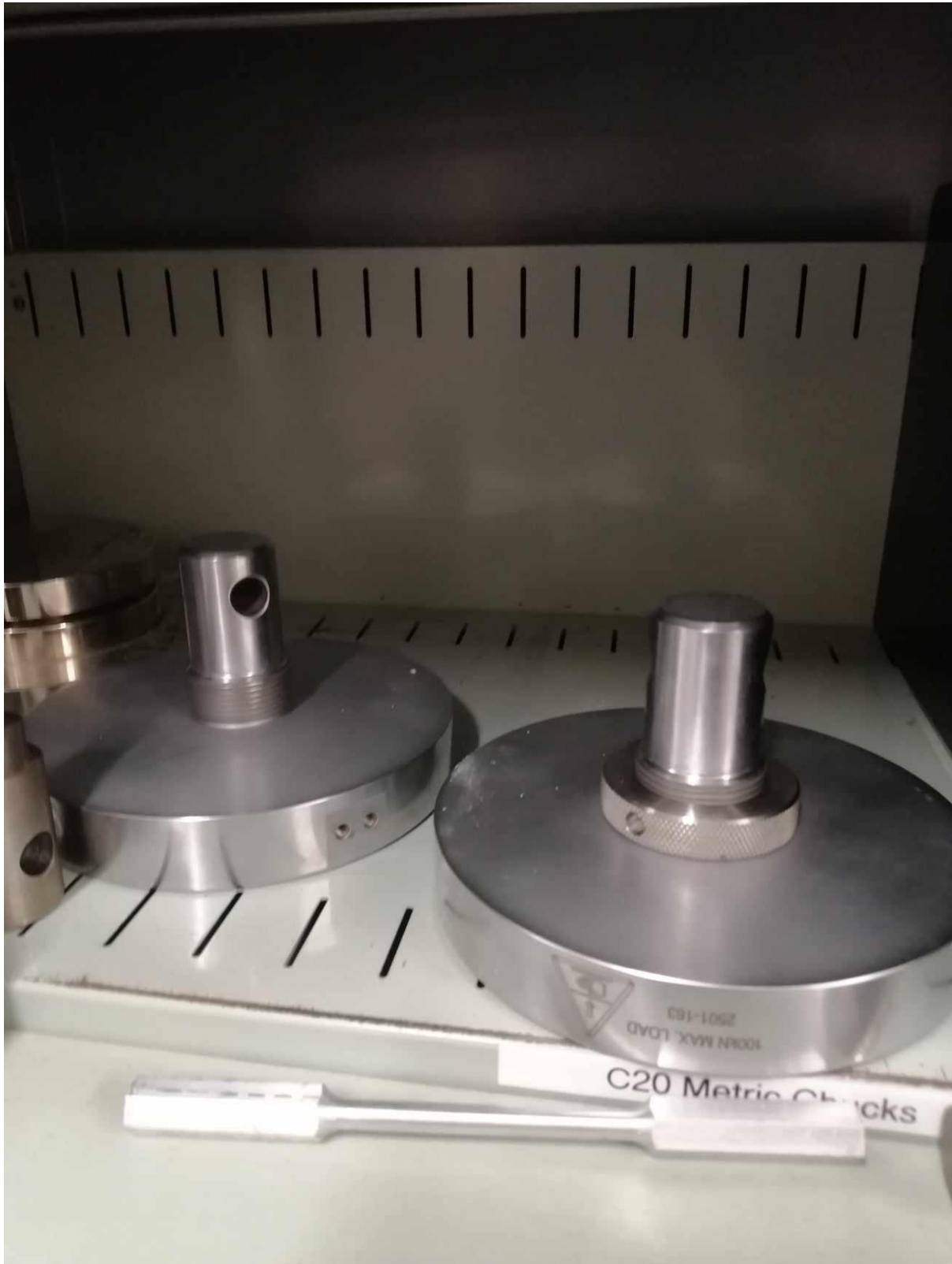
Figure 35: Loading platens used for compression test
