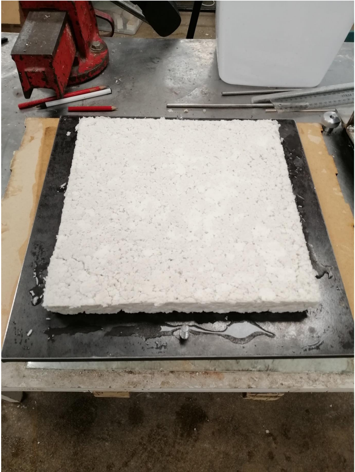
Figure 14: Removing large panel from mould, ready for drying.
