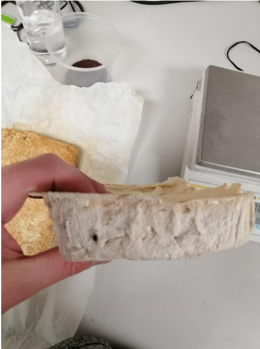
Figure 23: Tapioca starch panel after removal from foil baking tray.
