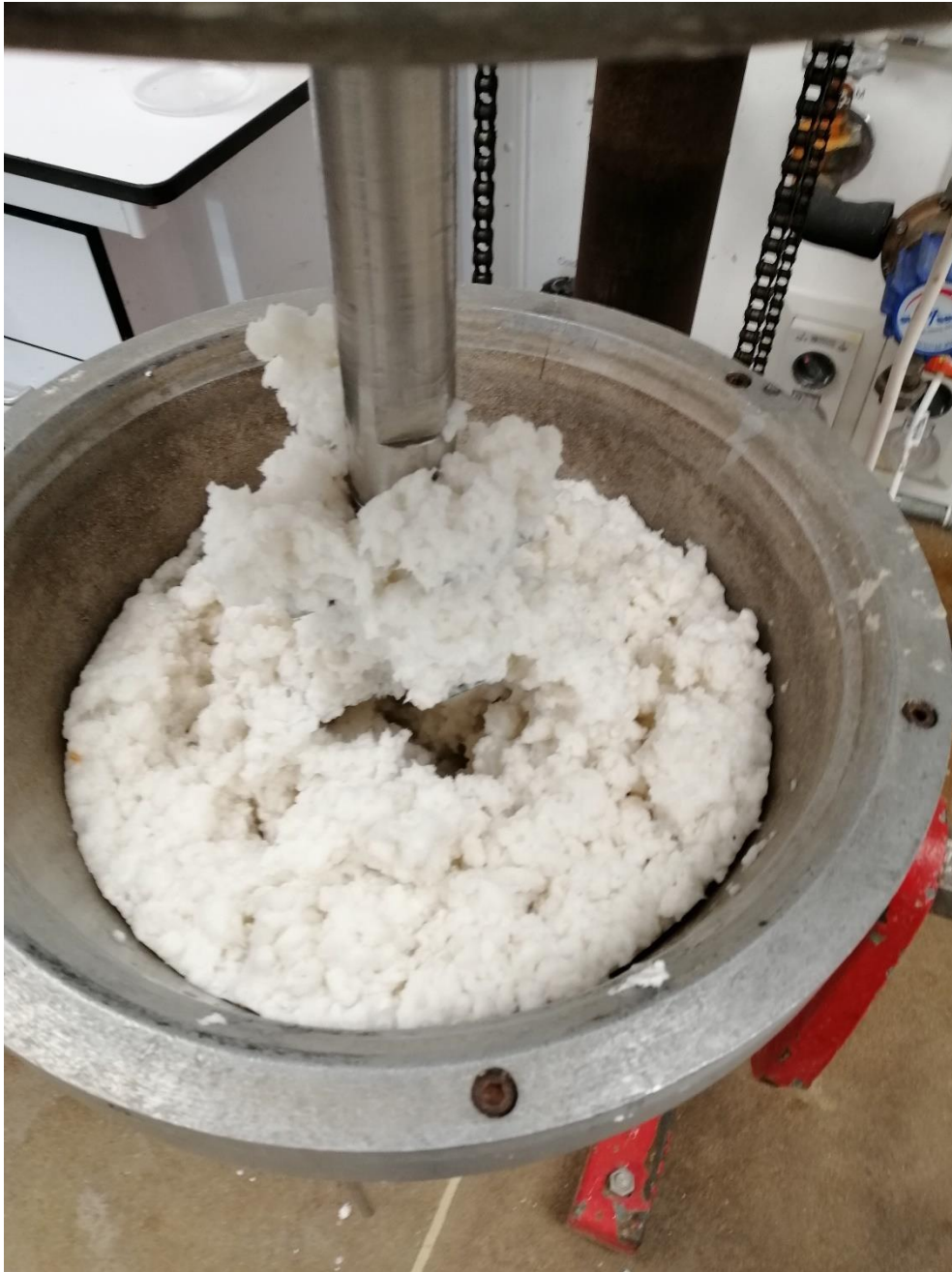
Figure 7: End of pulping in wet disintegrator.
