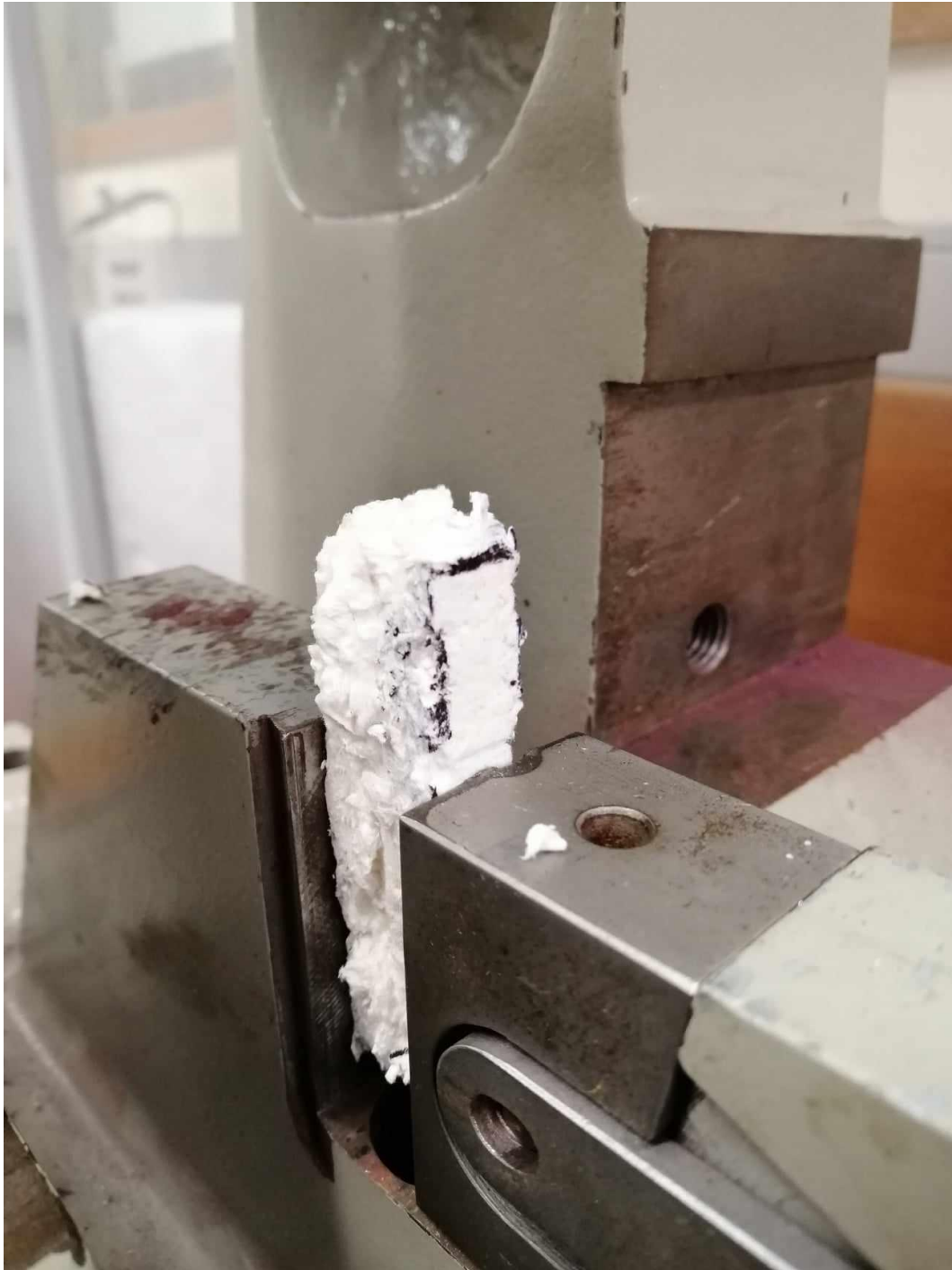
Figure 59: Pulp sample loaded in testing rig before impact
