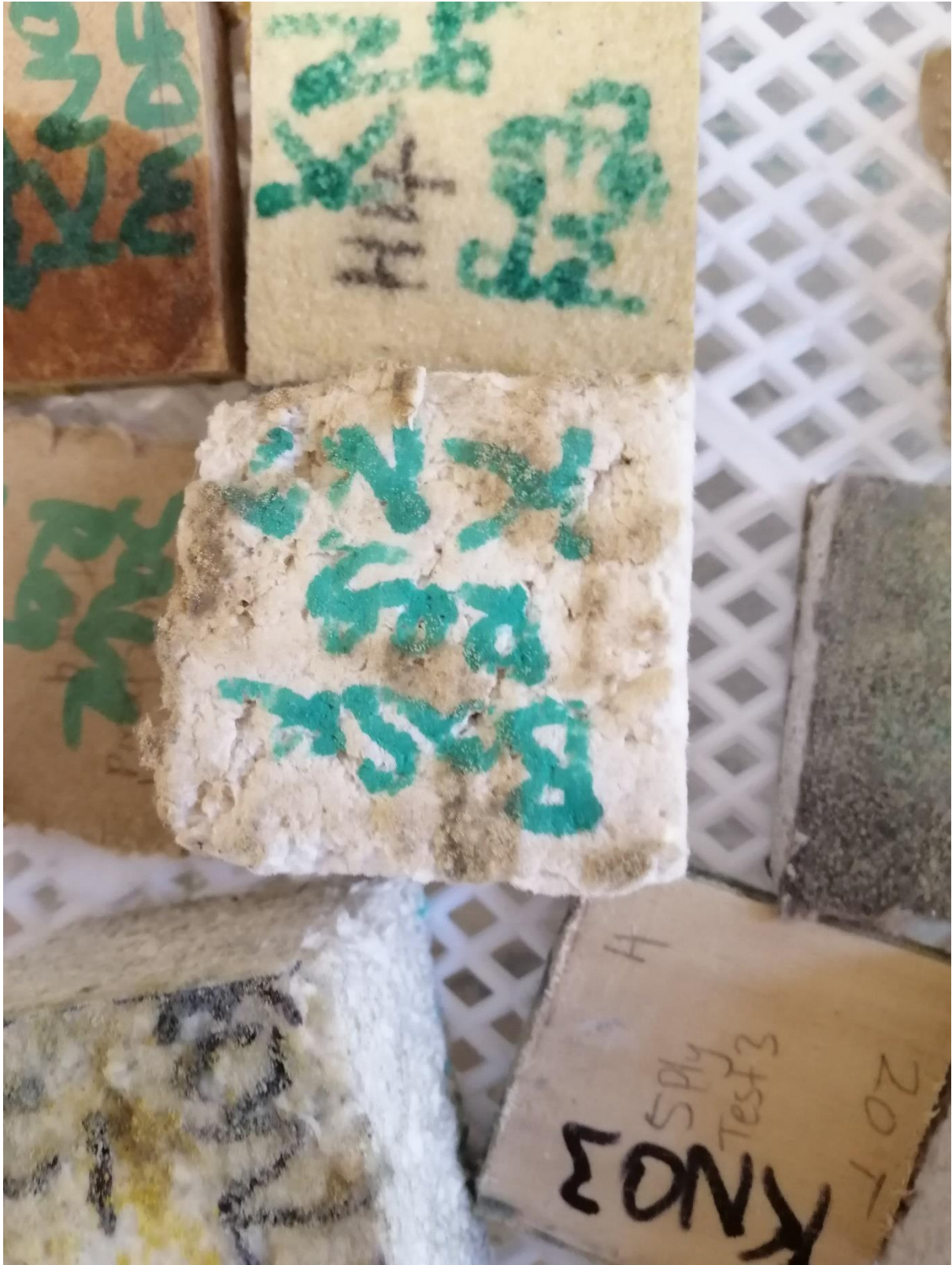
Figure 43: Close up of regular panel (just pulp) after exposure to \text{KNO}_3
