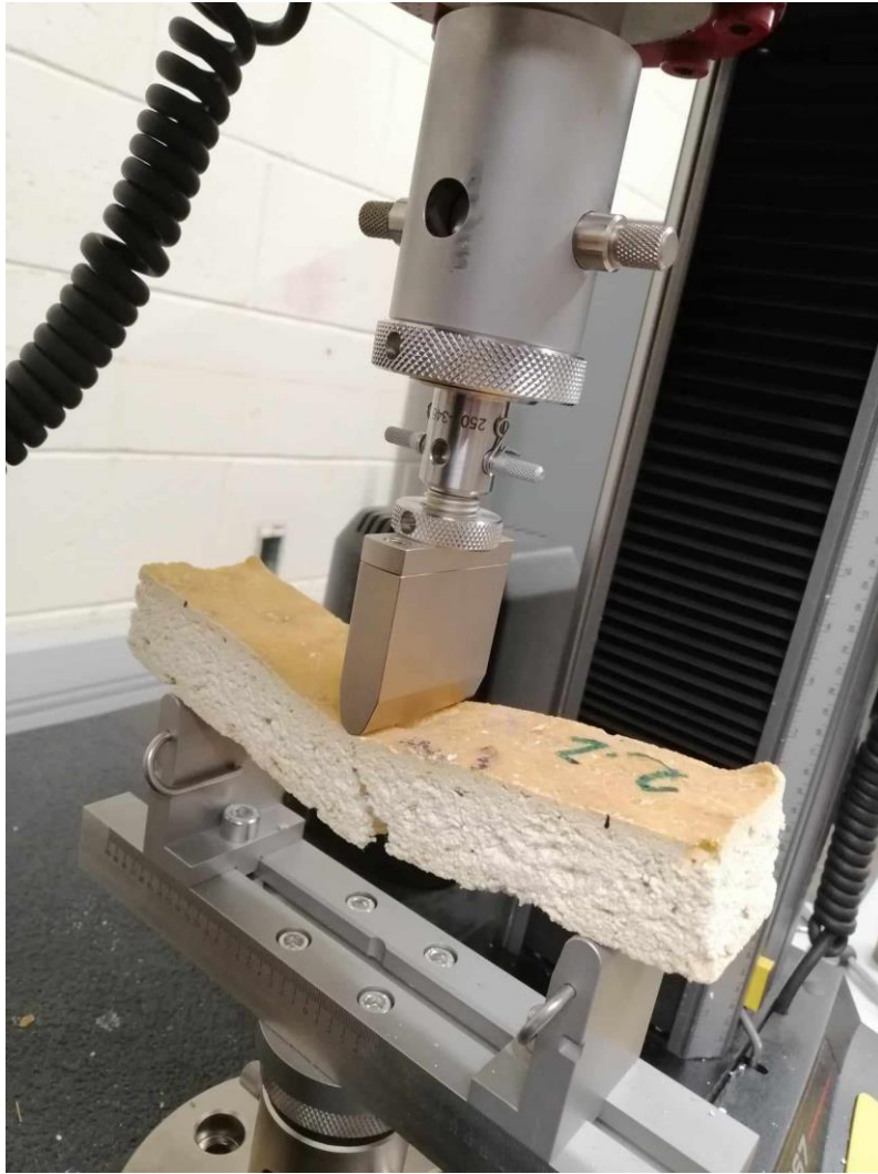
Figure 57: Bending test on casein panel sample
