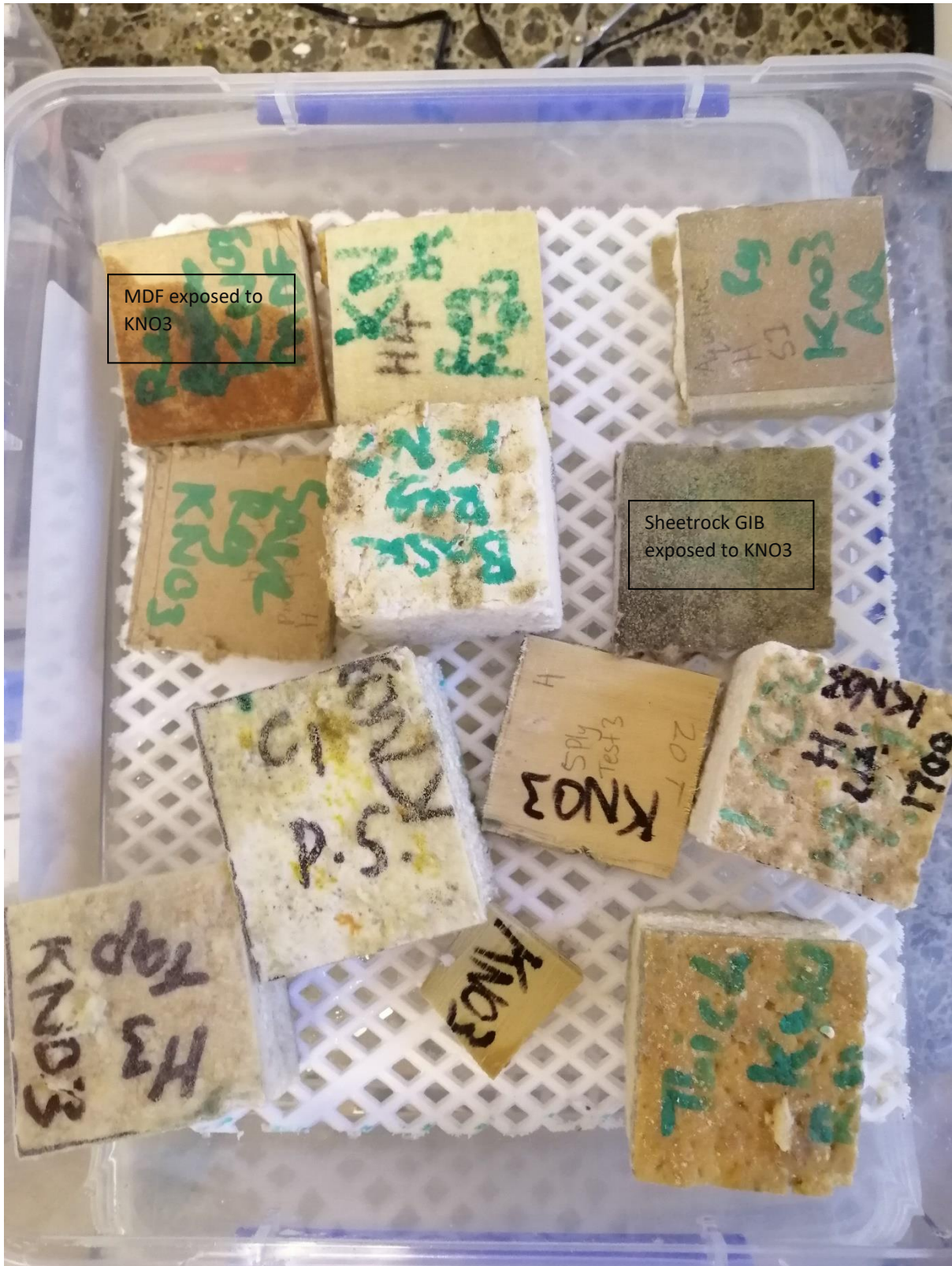
Figure 40: Specimens exposed to KNO_3
