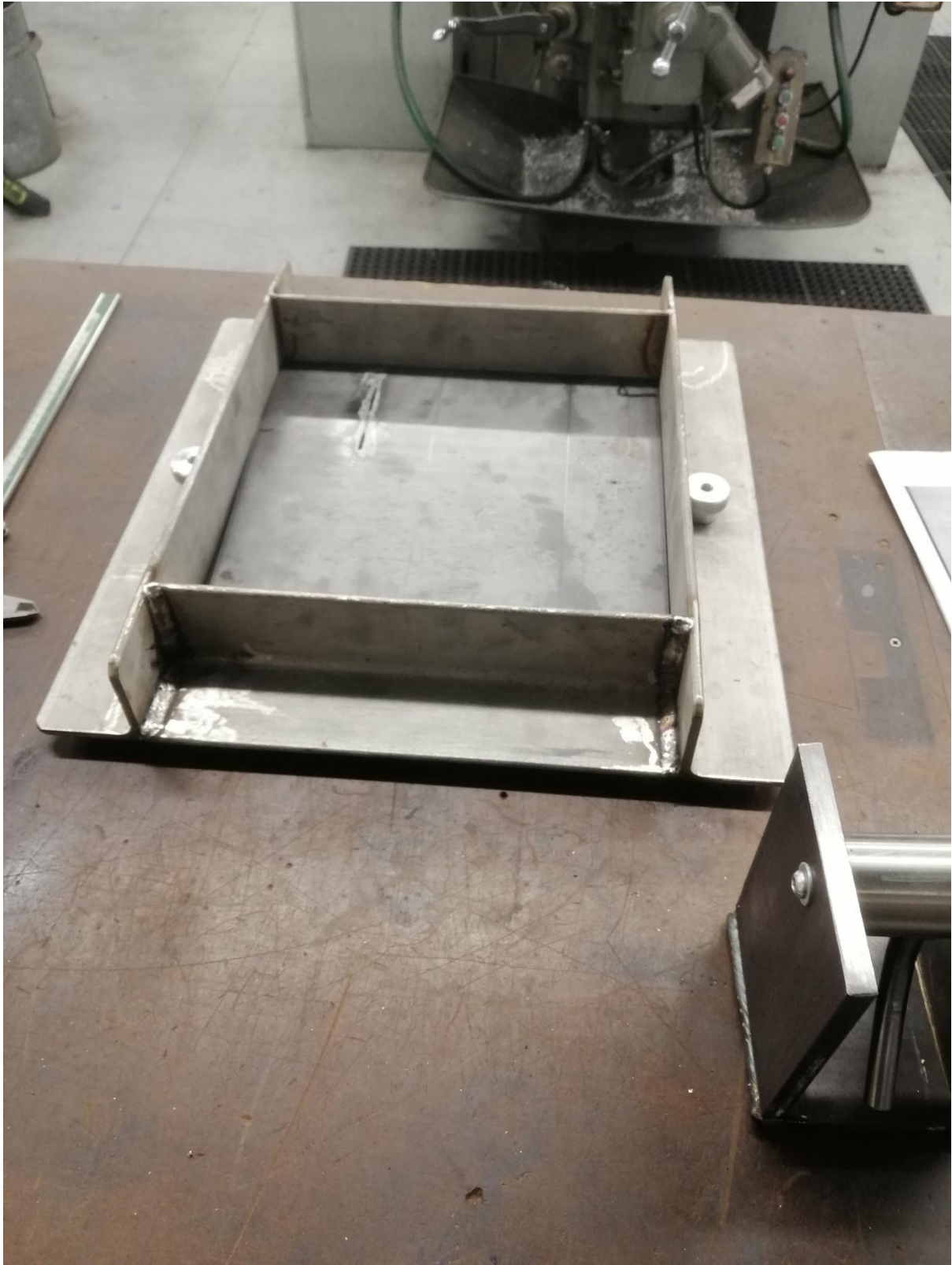
Figure 12: Large mould used for making big panels (before painting).
