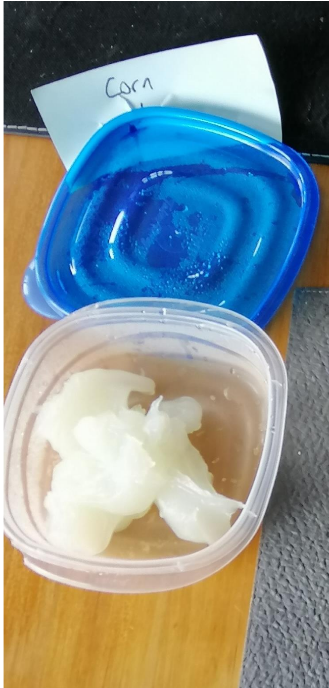
Figure 20: Solidified corn starch glue.
