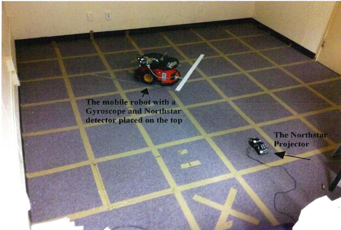
Figure 28: Testing the completed localization system with the mobile robot
