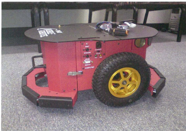
Figure 10: The Pioneer3-DX mobile robot used in this project
