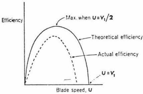
Figure 8.7 Relationship between Blade Speed and Efficiency (Massey, 1970)
