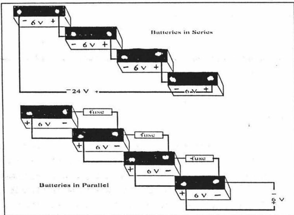
Figure 4.6 Series and Parallel Battery Configurations (Ministry of Energy, 1986)
