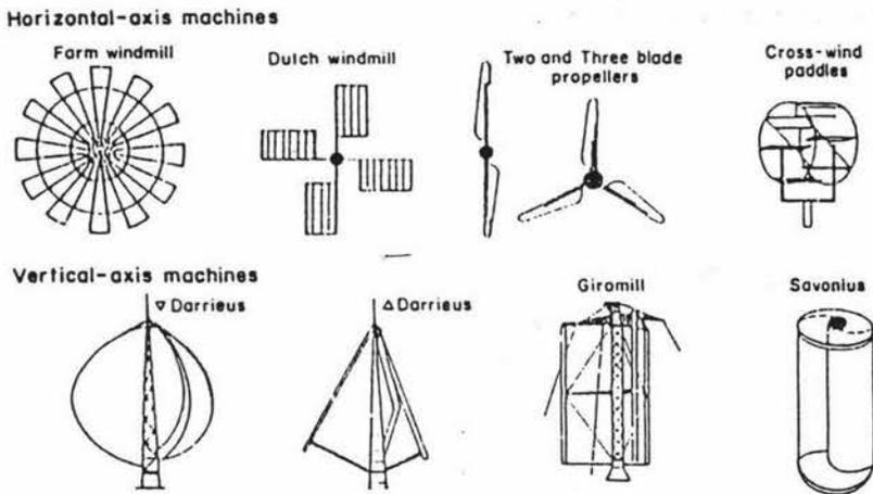
Figure 7.7 Common Types of Wind Turbine
