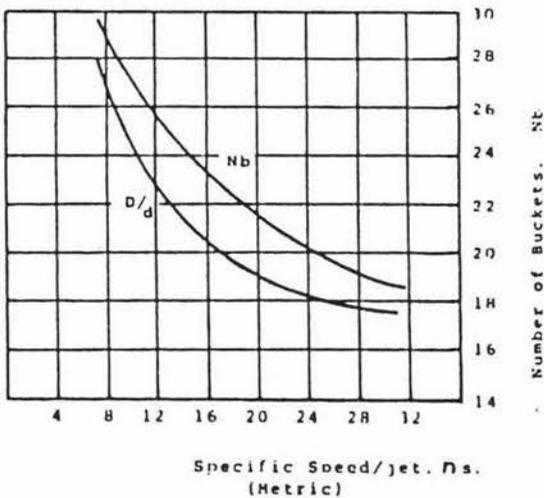
Figure 8.6 Specific Speed Relating to Number of Buckets (reproduced from MAF Aglink, AST 65/7)
