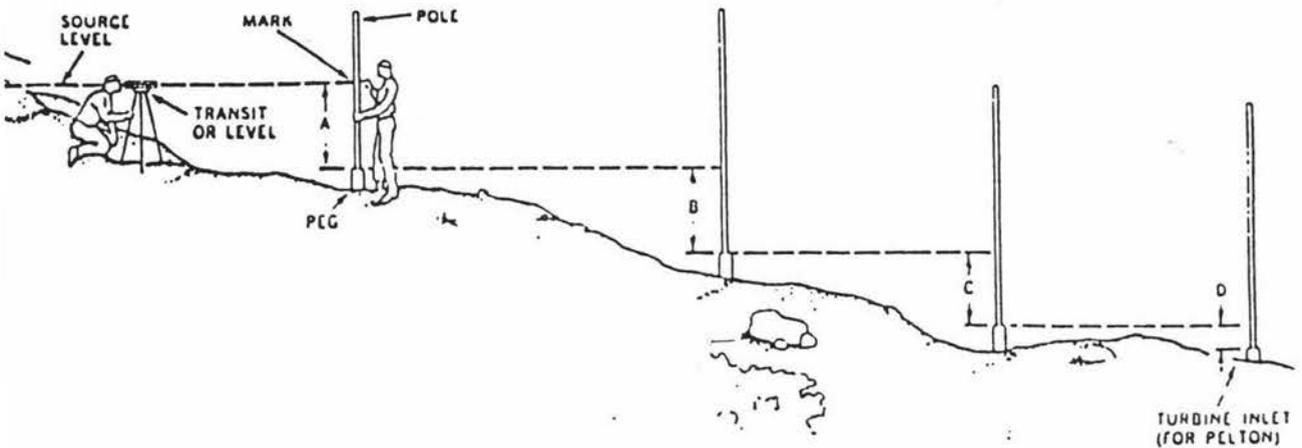
Figure 8.2 Measuring Head using Surveying Equipment (Tamar Designs)
