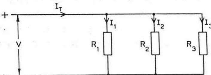
Figure 4.1 A Parallel Circuit (New Zealand Technical Correspondence Institute, 1977)
