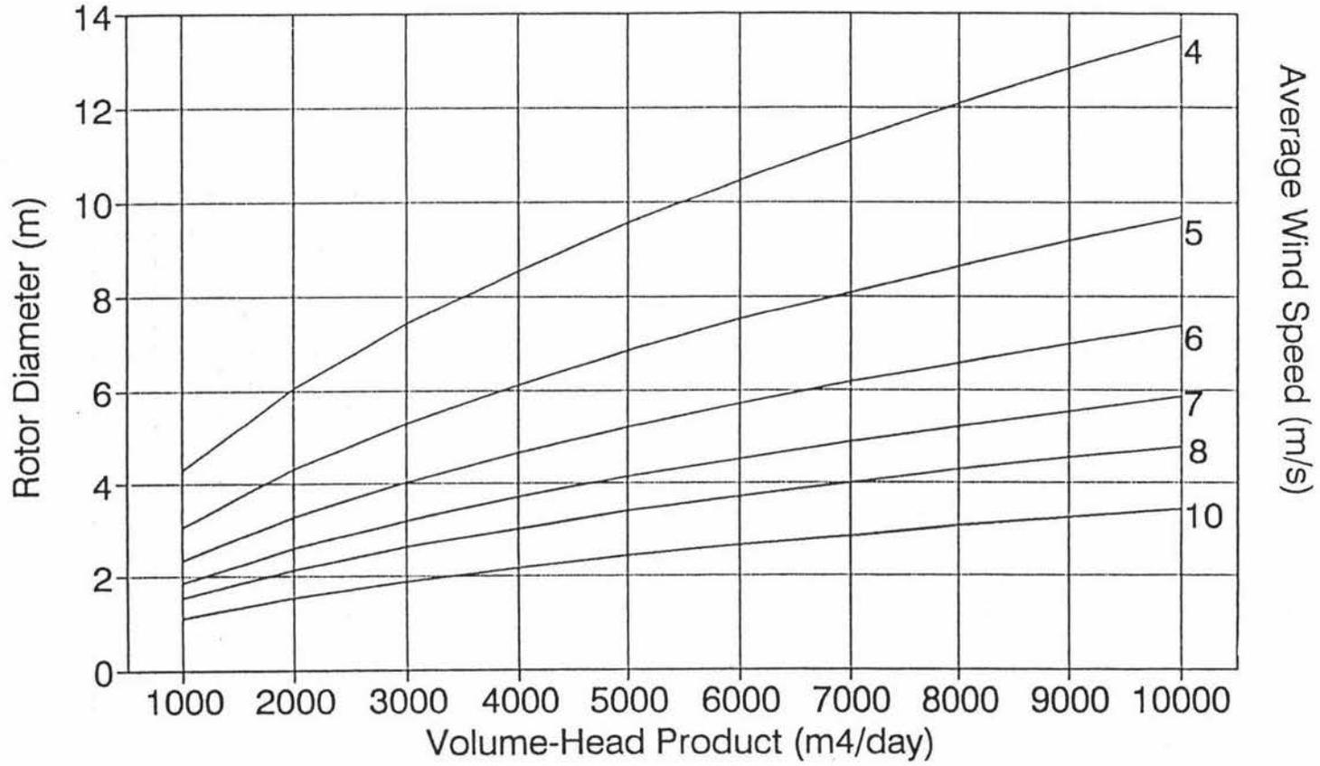
Figure 7.13 Nomogram for Sizing Wind Pump Rotor (EPF 1.9)
