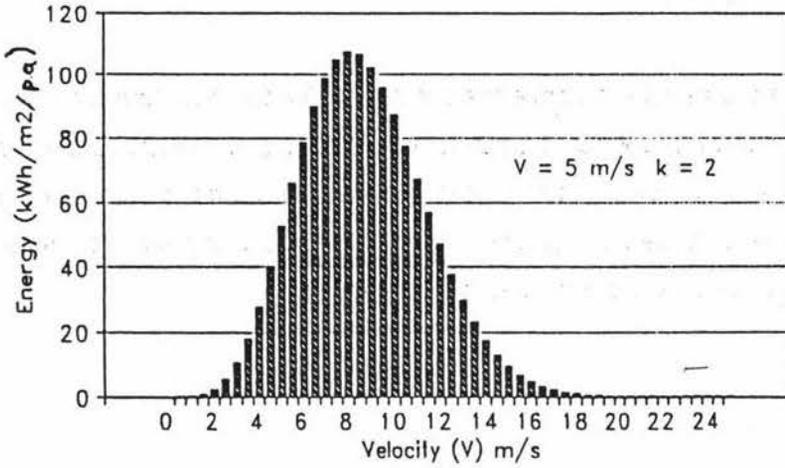
Figure 7.10 Wind Power Duration Curve
