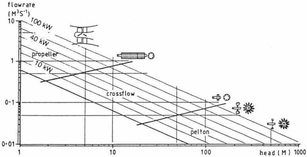
Figure 8.3 Turbine Selection Chart for Relatively High Flows (Adapted from Hothersal, 1984)
