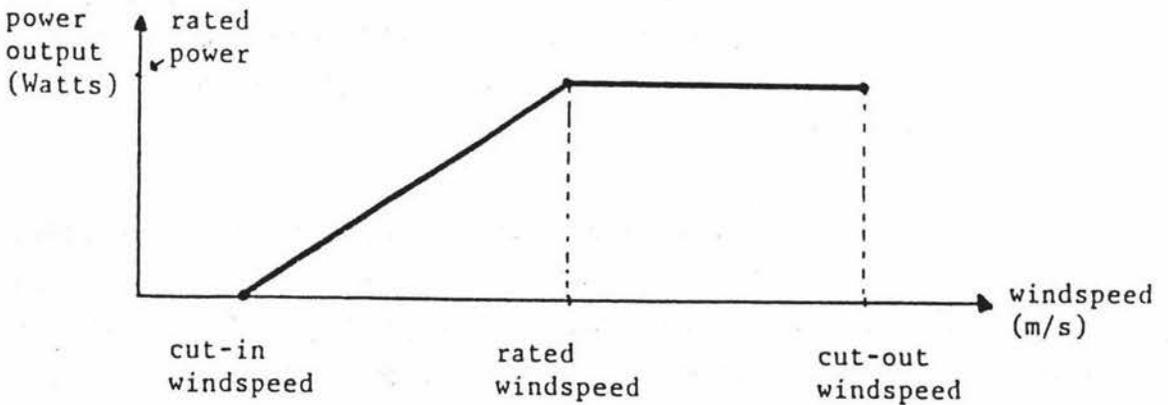
Figure 7.11 Standard Turbine Output Curve
