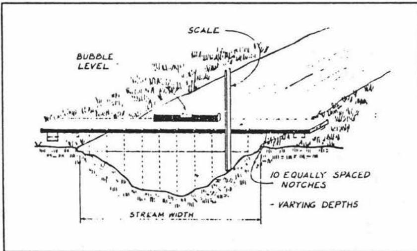
Figure 8.1 Measuring Flow with a Float (Ministry of Energy, 1986)
