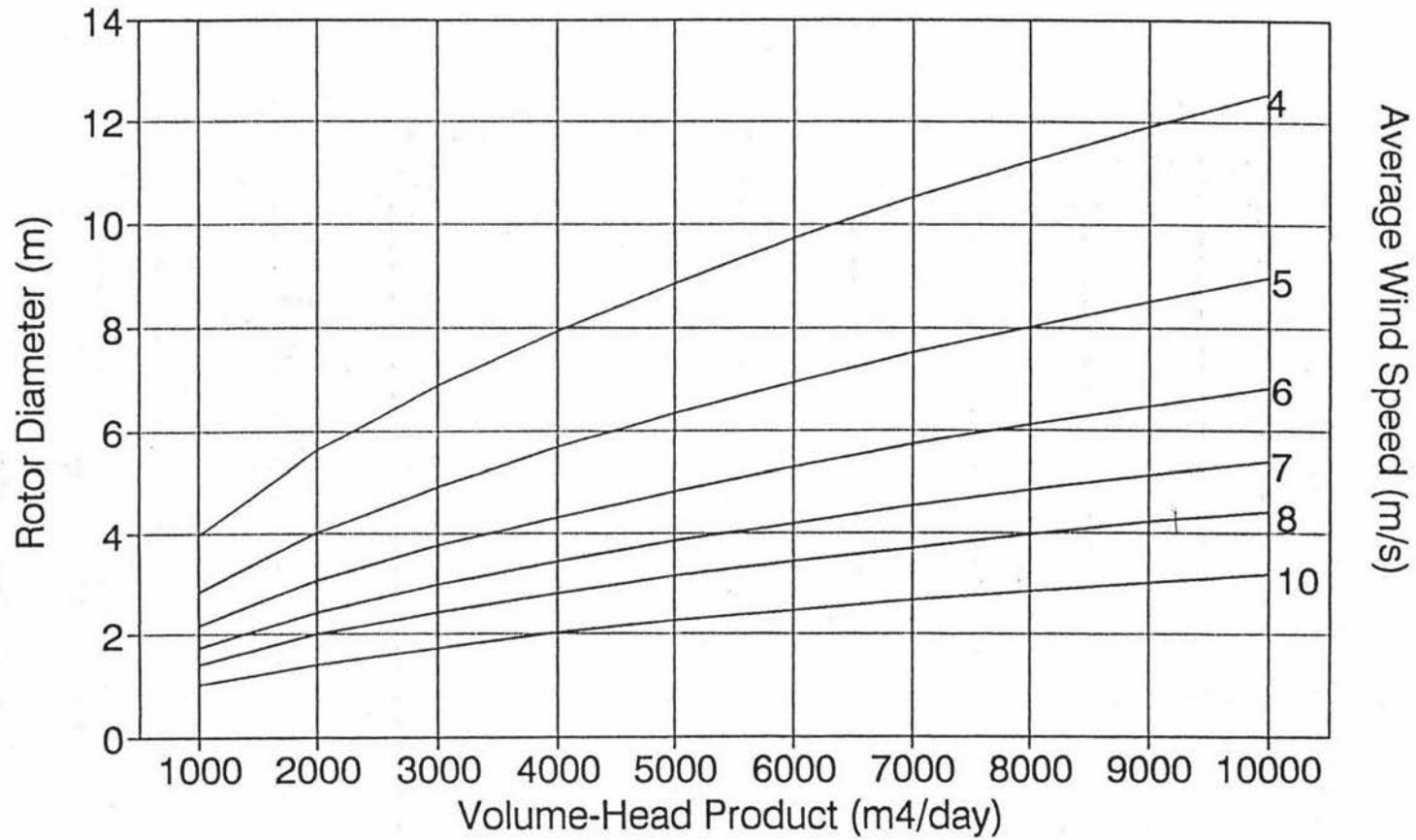
Figure 7.14 Nomogram for Sizing Wind Pump Rotor (EPF 2.2)
