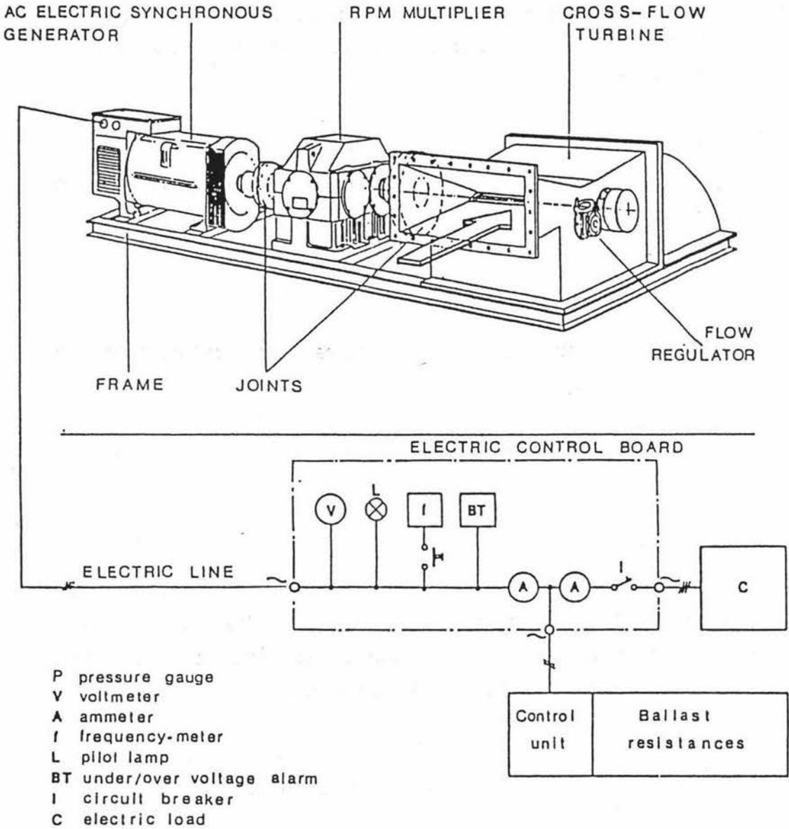
Figure 8.13 Crossflow Turbine Electricity Generating System (adapted from the 'Ecowatt' product manual)
