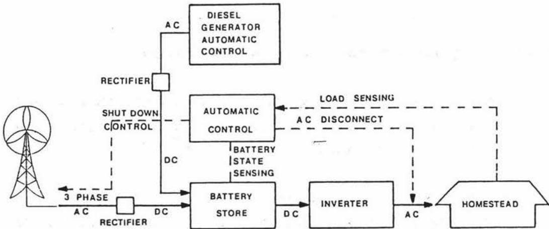
Figure 9.3 Hybrid Wind-Diesel Electric Power System (Edwards, 1986 - adapted from Langworthy, 1984).
