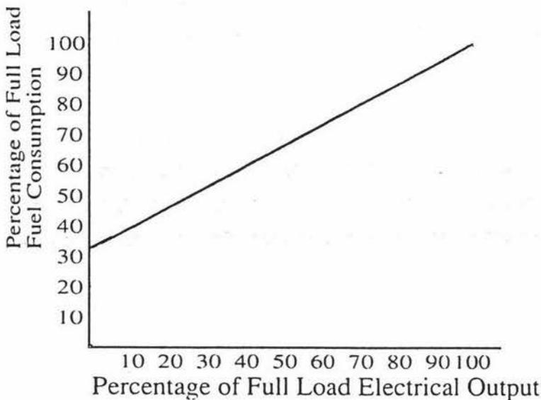
Figure 9.2 Fuel Usage versus Electrical Load (Adapted from Lipman, 1988).
