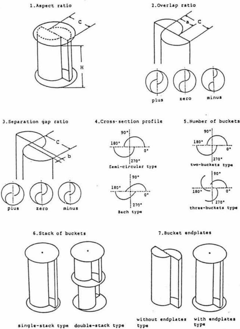
Figure 7.8 Savonius Rotor Design Parameters (Nahas et al, 1987)
