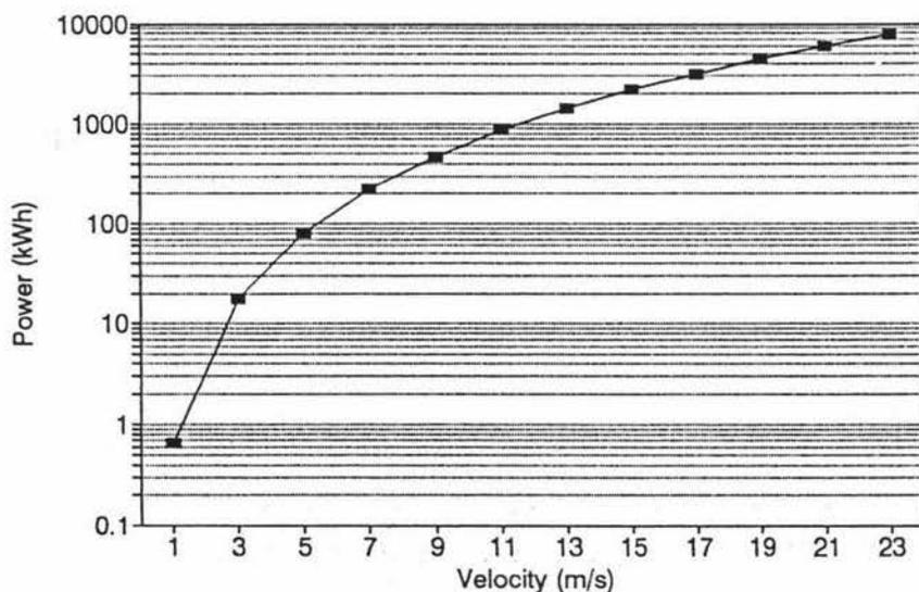
Figure 7.1 Relationship between Velocity and Wind Power
