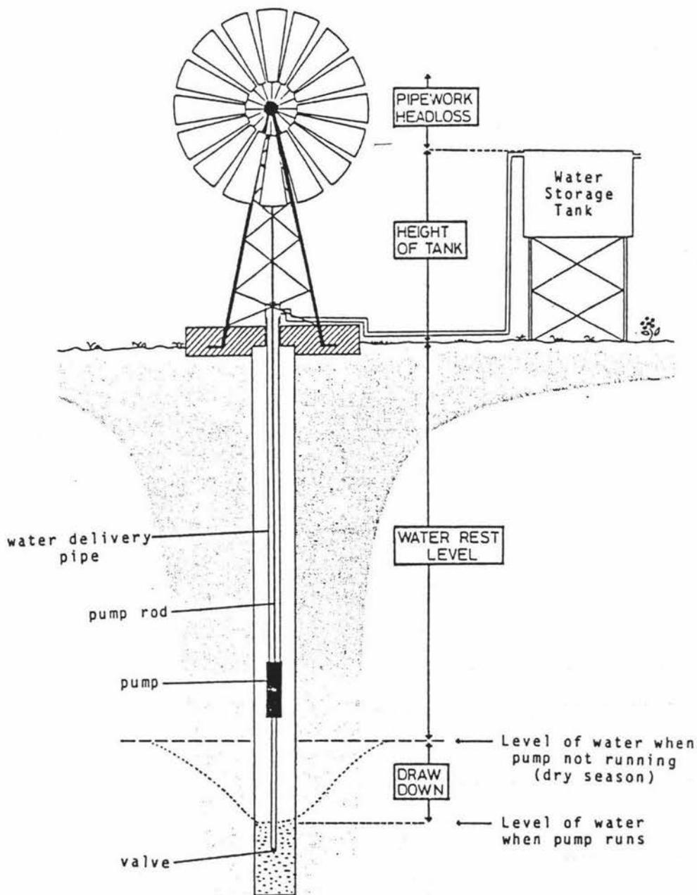
Figure 7.12 Schematic Representation of Wind Pumping Head Components (Lancashire et al, 1987)
