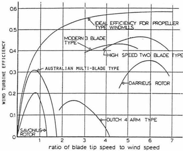
Figure 2.1 Efficiency versus Tip Speed Ratio (Dunn, 1986)
