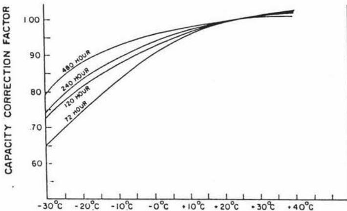
Figure 4.5 Battery Capacity Correction for Temperature (Lasnier & Ang, 1990)
