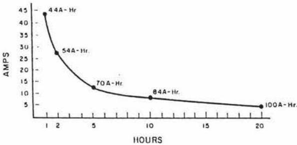
Figure 4.7 The Relationship Between Ampere-hour Capacity and Discharge Rate (Exide Battery Promotional Material)
