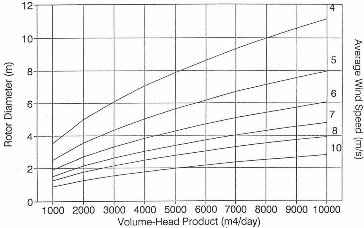
Figure 7.15 Nomogram for Sizing Wind Pump Rotor (EPF 2.8)
