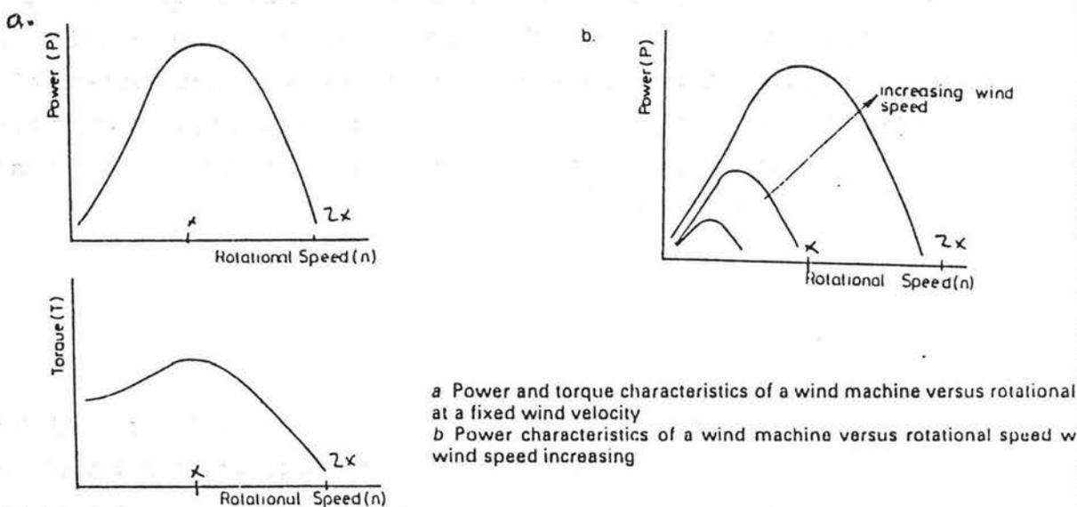
Figure 2.2 Power and Torque versus Rotational Speed (Dunn, 1986)
