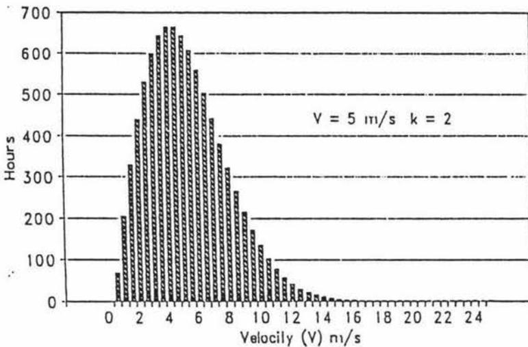
Figure 7.9 Wind Speed Frequency Distribution
