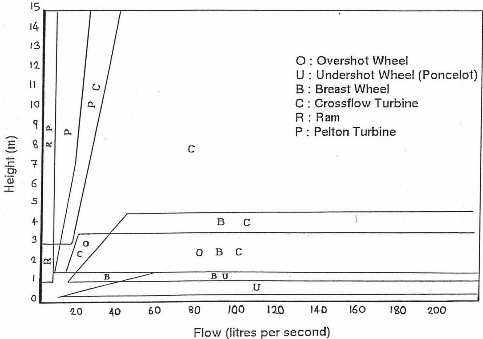
Figure 8.4 Turbine Selection Chart (adapted from Dakers & Martin, 1982)
