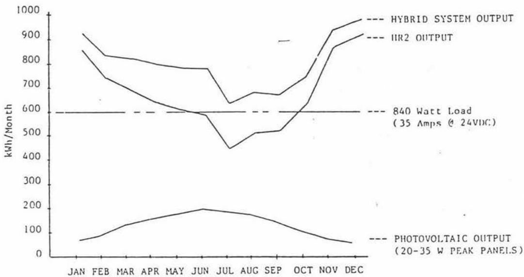
Figure 9.1 Turbine Output showing Photovoltaic Contribution (Mayer, 1985)
