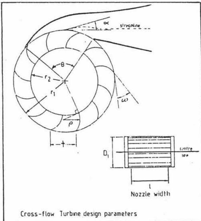
Figure 8.8 Crossflow Turbine Design Parameters (Dakers and Martin, 1982)
