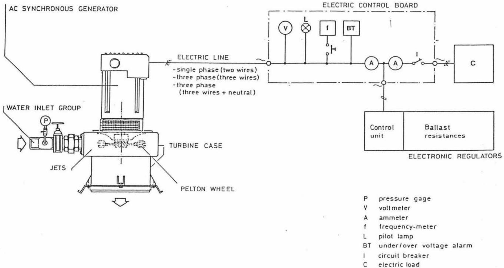
Figure 8.12 Pelton Wheel Electricity Generating System (adapted from 'Ecowatt' product manual)
