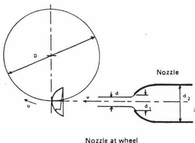
Figure 8.5 Pelton Wheel Design Parameters (MAF Aglink, AST 65/7)
