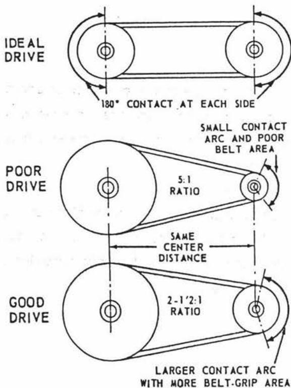
Figure 4.8 The Effect of Pulley Size on Drive Suitability (John Deere, 1980)
