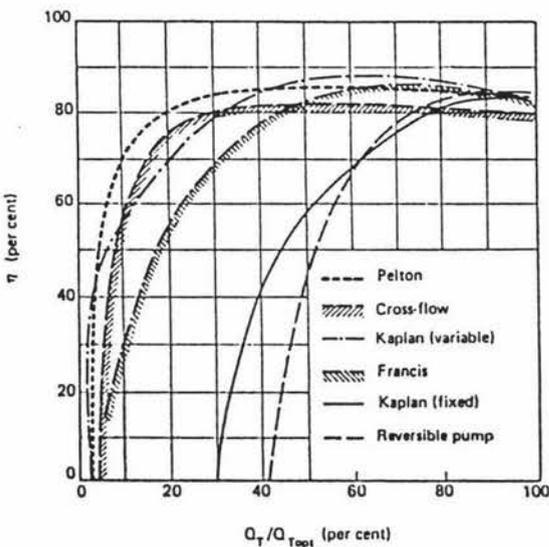
Figure 8.9 The Relative Performance of Turbines Measured Against Percentage of Design Flow (Engeda & Rautenberg, 1988)
