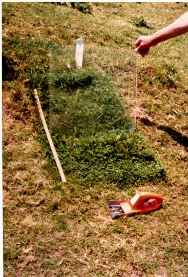
Plate 4.3 Pasture on a 25° slope plot prior to harvest 29 days following isotope placement. Perspex sheet in position to shield operator from the "hot line" and battery-powered harvesting shears ready for use.
