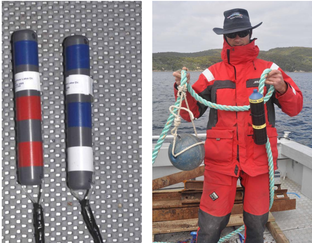
Figure 2. 2 - Acoustic tag and receiver. Left: Vemco V16-5H R-code acoustic tag. Right: Vemco VR2W acoustic receiver attached to mooring prior to deployment northeast of Stewart Island, New Zealand. Photos: Malcolm Francis.
