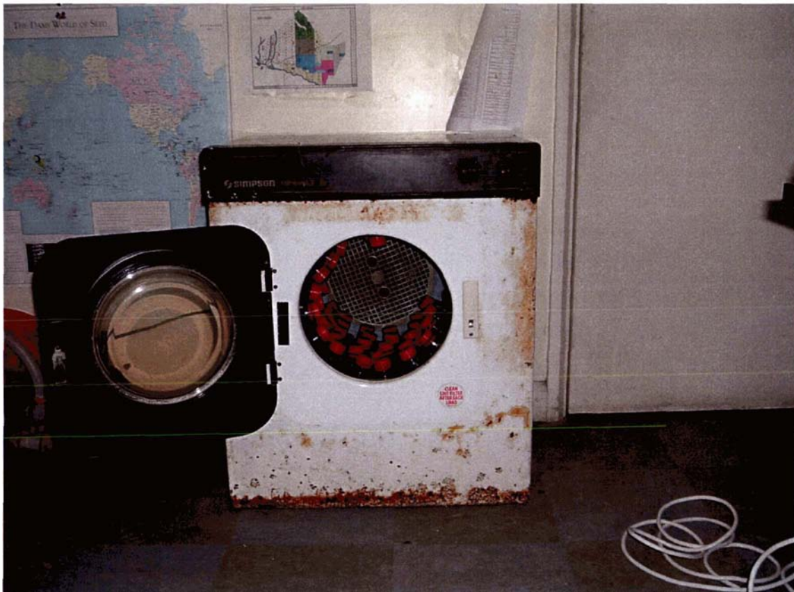
Plate 5.1 Modified clothes drier used as end-over-end shaker for extractions
