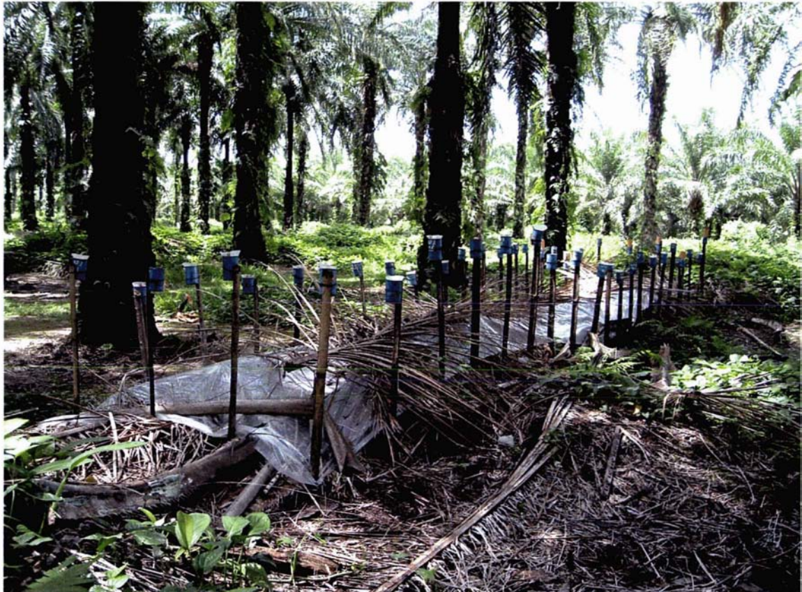
The blue catch cans on the stakes were used for estimating throughfall
