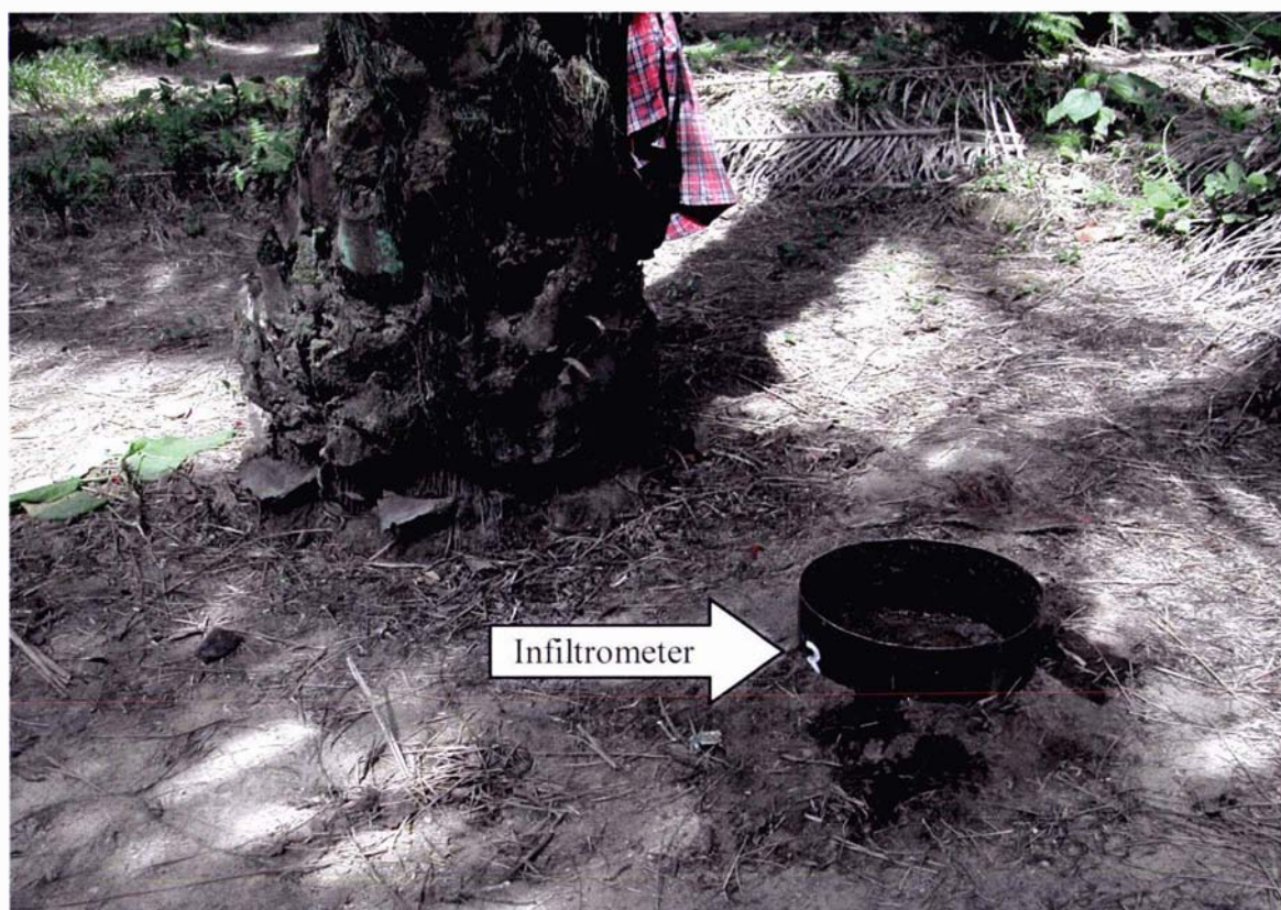
Plate 4.1 Inserted infiltrometer in the weeded circle
