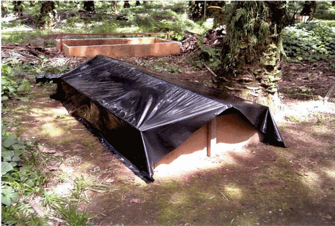
Plate 5.3 Plastic cover to prevent throughfall from reaching the plots
