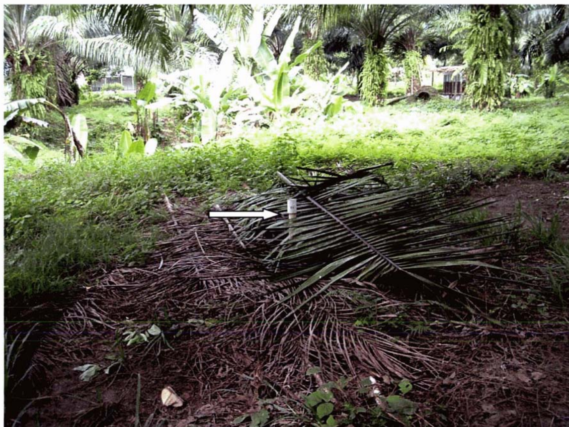
Plate 8.1 A suction cup installed in a frond pile at Sangara, showing an empty can capping the pvc pipe
