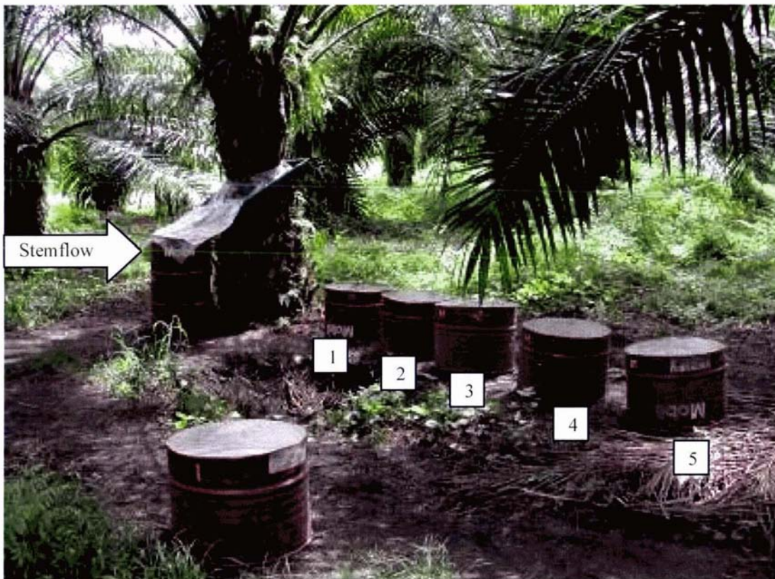
Plate 4.2 Throughfall drum numbers 1 – 5 and stem flow field set-up
