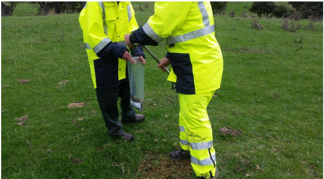
Figure 26 Combining soil samples to be sent for wet chemistry laboratory analyses
