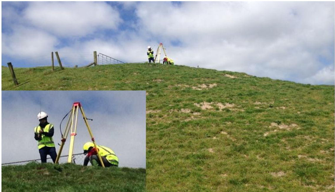
Figure 20 Setting up the Leica RTK-GPS base station
