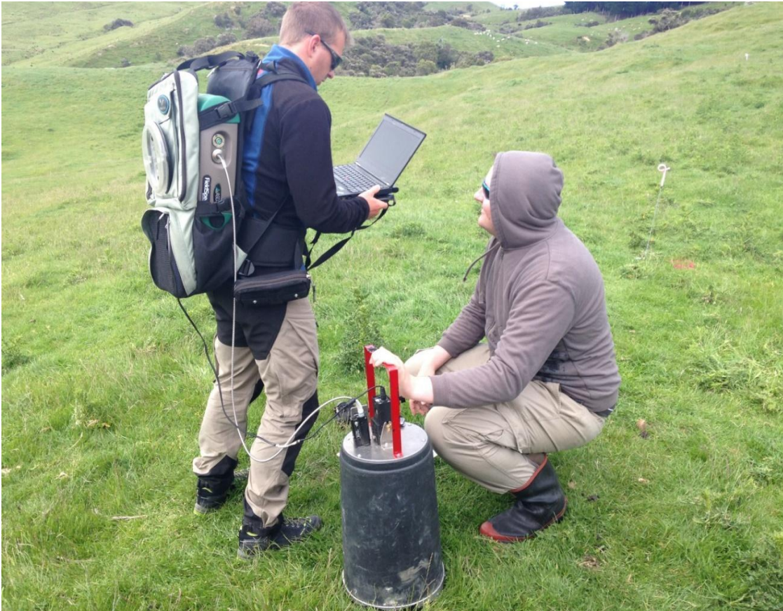
Figure 24 P2P team members use the ASD to collect proximal hyperspectral data at Farm 5
