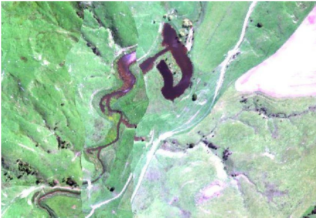
Figure 29 Image with poorly aligned image strips
