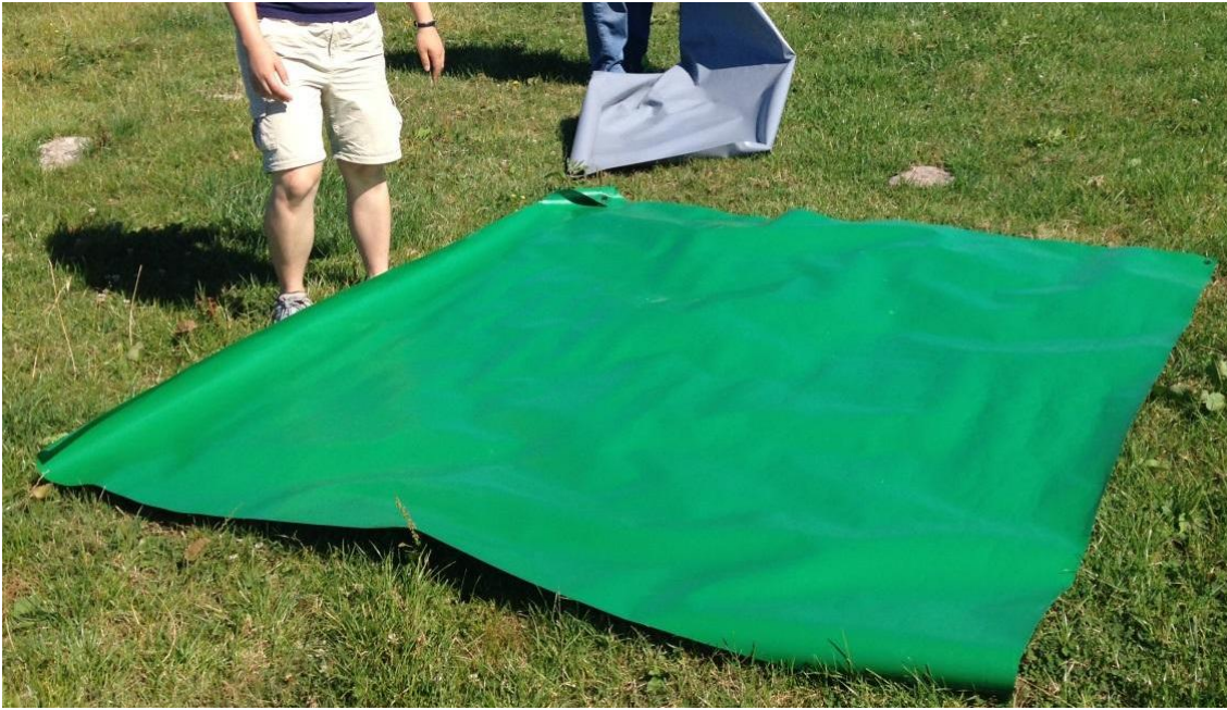
Figure 31 Researcher positioning a reference tarpaulin employed for georectification purposes
