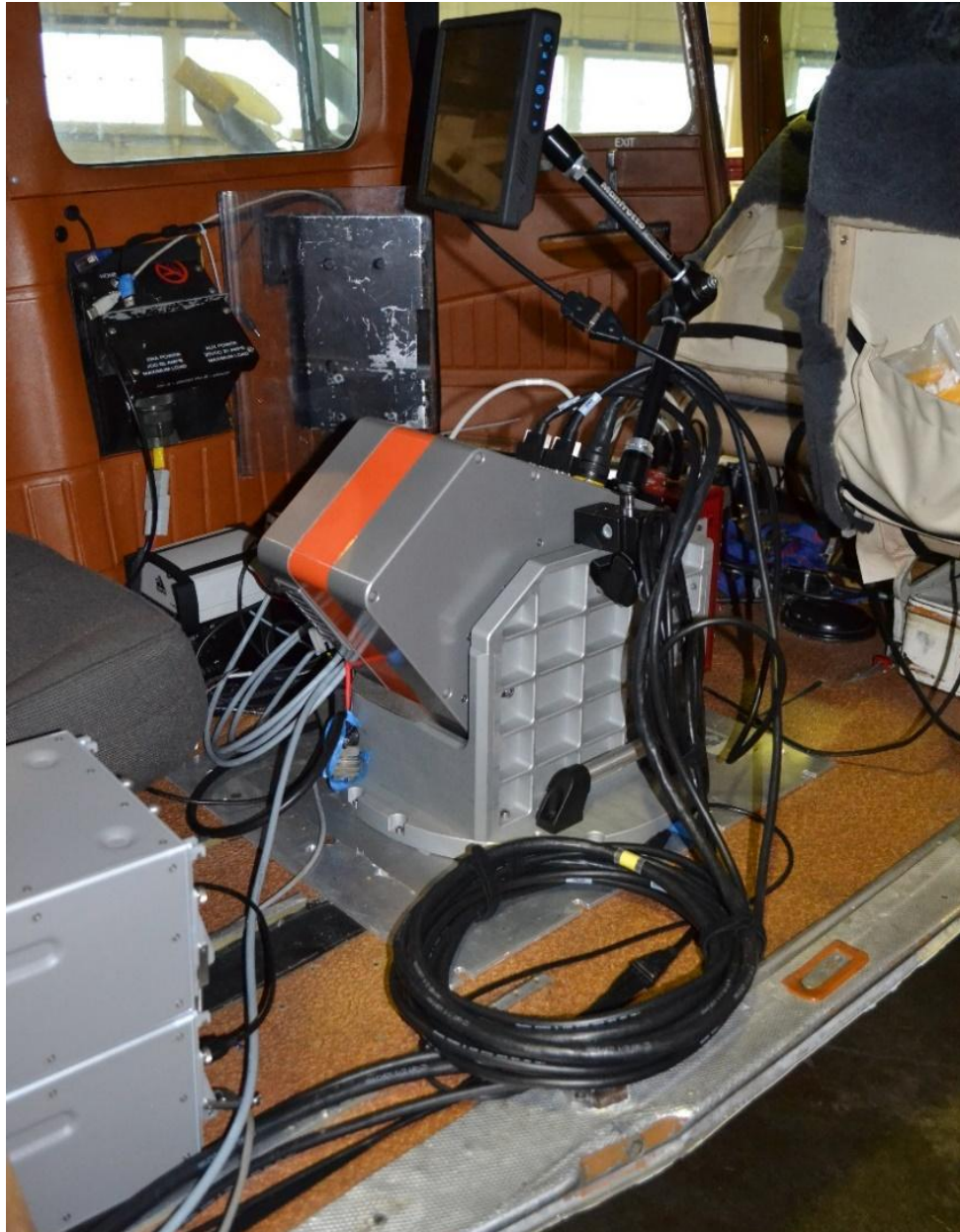
Figure 16 Massey University's AisaFENIX installed in a survey aircraft. Source: Aerial Surveys Ltd
