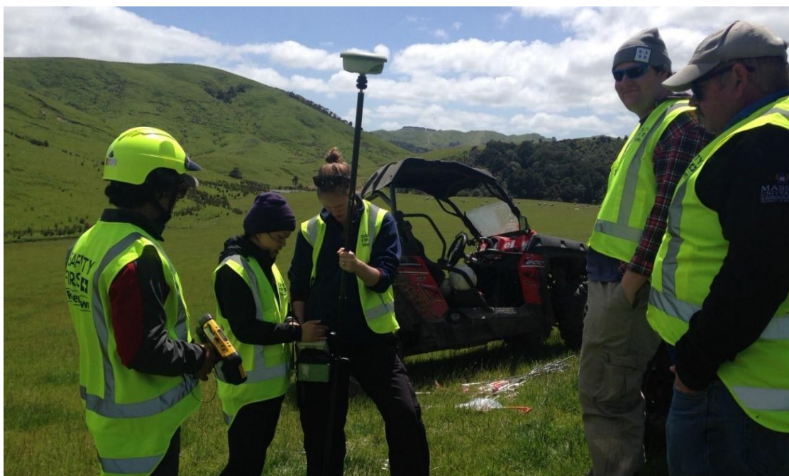
Figure 21 P2P researchers geolocate permanent marker locations using Leica RTK-GPS
