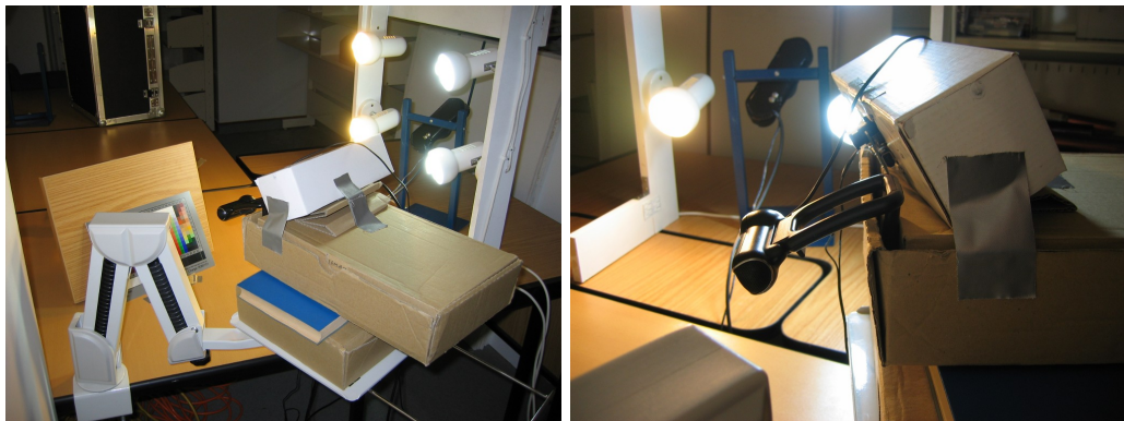
Figure 8.2: Setup of sampling assembly for the colour shift sample analysis series. (left) Geometric arrangement of the colour test chart, light fixture (for the case “65652727”) and cameras. (right) The cameras are mounted into a fixed position to ensure equal an capturing arrangement for all illumination cases.
