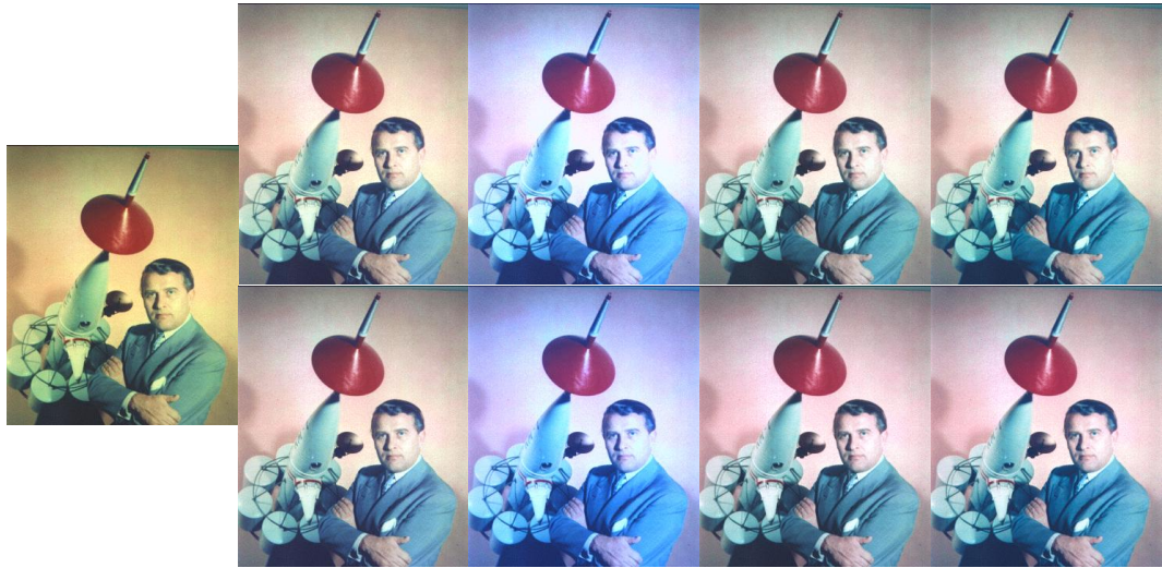
Figure 4.7: (left) Original 1950’s picture of Wernher von Braun. (top row) Colour corrected according to Grey World Assumption. (bottom row) Colour corrected according to White Patch Retinex algorithm. Chromatic transformations (left to right): RGB channel scaling, RGB with Bradford transformation, L^*a^*b^* with channel scaling, L^*a^*b^* with Bradford transformation.
