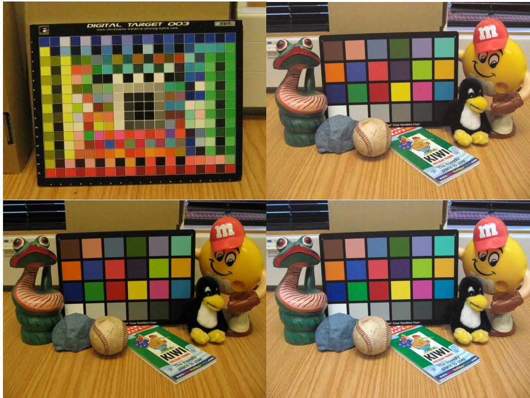
Figure 7.6: (top left) Uncorrected image captured of test chart used for computing the ICC profiles. (bottom left) Uncorrected RGB image as taken by the camera. (top right) Colour corrected image using the ICC profile by our profiler Mārama. (bottom right) Colour corrected image using an ICC profile created by Argyll CMS.
