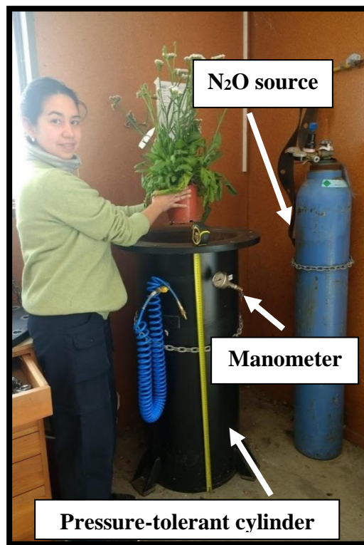
Figure A-6 Equipment utilised for treating plants with nitrous oxide ( N_2O ), which included a pressure-tolerant cylinder (inside diameter 45 cm; height 110 cm), a N_2O source, and a manometer. Photo taken by Steven Ray.
