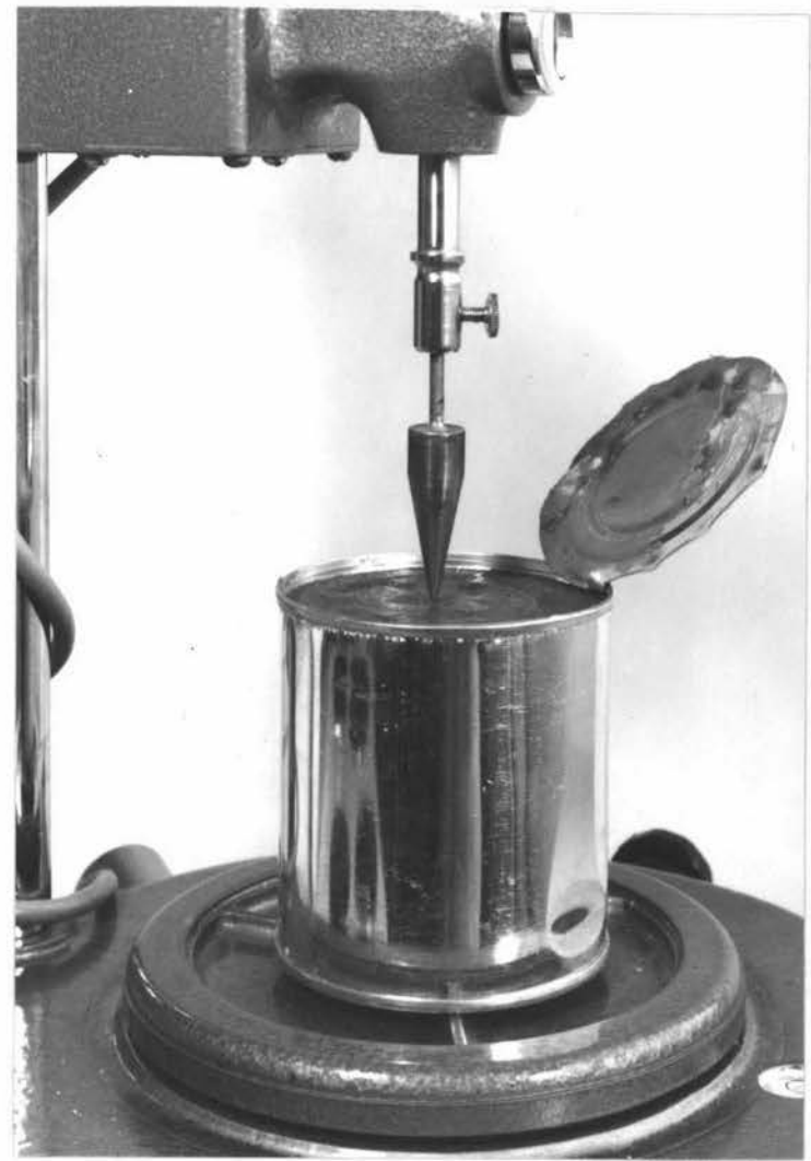
FIGURE 25. 'CENTRAL' penetrometer model used for the determination of the gel strength of caramelized sweetened condensed milk. Both the complete unit (left) and a closer view of the type of plunger used (right) are shown.
