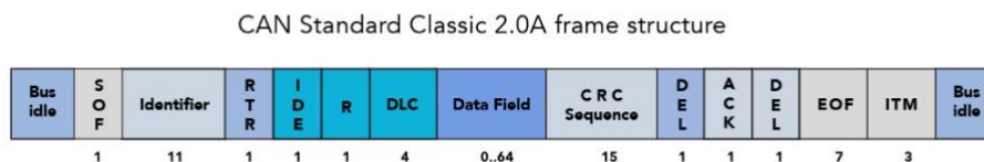
Figure 22 Can Standard Classic 2.0A Frame Structure
