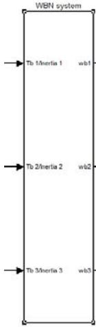
This block represents the angular velocity of the satellite, we can see that torque from magnetic coils is one of the main components for this block of the system, and it's logical as the angular velocity changes with amount of torque applied.
