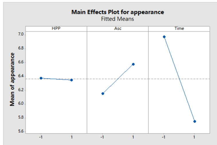
Figure 5.8 Factorial analysis of appearance with factors including Asc (level -1 represents no ascorbic acid and level 1 represents the incorporation of 2% of ascorbic acid), HPP (level -1 represents no HPP treatment and level 1 represents the HPP treatment at 600 MPa for 5 min) and time (level -1 represents storage time at week 0 and level 2 represents storage time at week 2).
