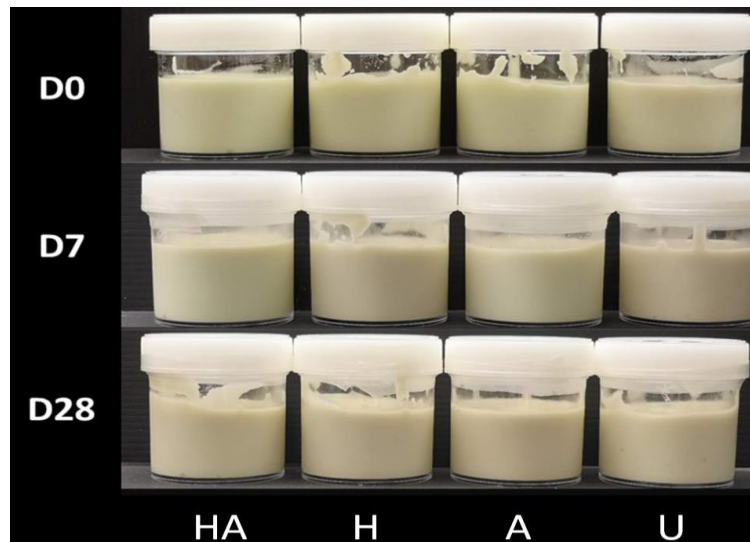
Figure 4.7 Colour change of yoghurt samples containing avocado that was untreated (U) or treated with HPP (H), 2% of ascorbic acid (A) and a combination of HPP and ascorbic acid (HA) during storage at day 0, 7 and 28.
