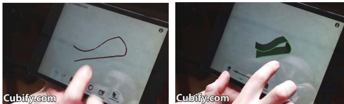
Figure 12. Cubify Draw allow a user to easily create an extruded design using touch input
