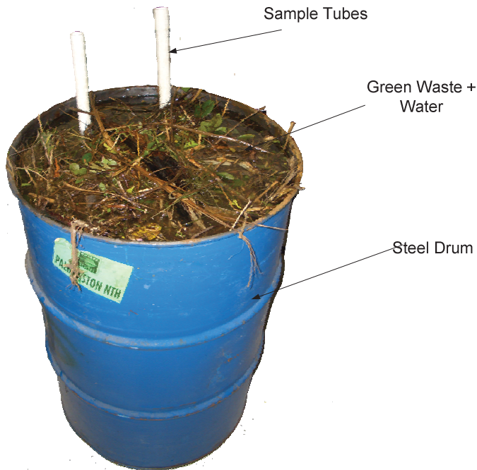
Figure 3.1: Laboratory leaching tank setup
