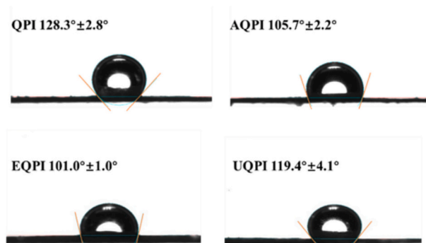
Fig. 4. The contact angle images of a water droplet on protein films in oil. QPI represents quinoa protein isolate; AQPI, EQPI and UQPI represent acid-hydrolyzed, enzyme-hydrolyzed, and ultrasonication-modified QPIs, respectively.
