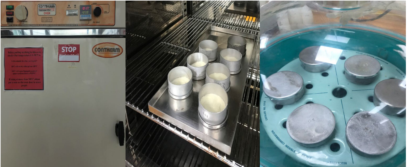
Figure 7: Gravimetric determination of Moisture Content Set-up
