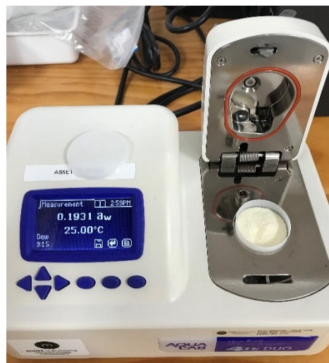
Figure 8: Water Activity Set-up
