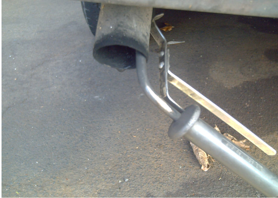
Figure 5-7 Tester Probe inside exhaust pipe
