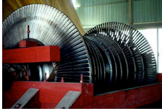
Figure 4-4 Turbine generator at geothermal power plant
