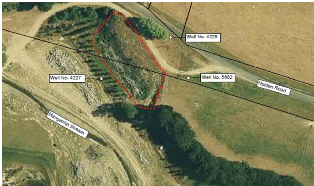
Figure 14: GIS map - Tikokino Closed Landfill - enclosed by the dotted red line indicates the extent of the former disposal area
