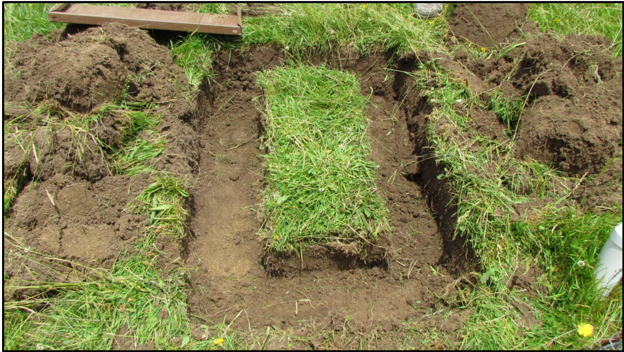
Plate 6.1 Collection of a soil slab from a point close to one of the C1North shallow slope runoff plots.
