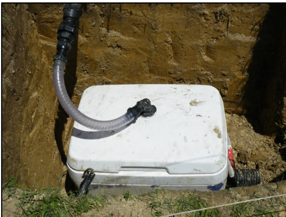
Plate 3.6 Surface runoff measurement system installed in the field.
