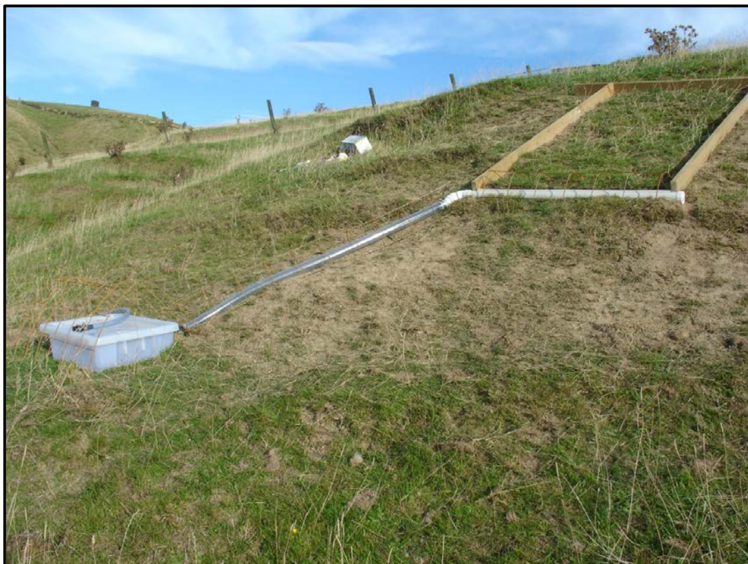
Plate 3.4 One of the C1 30 N plots showing the split PVC pipe and collection bin.
