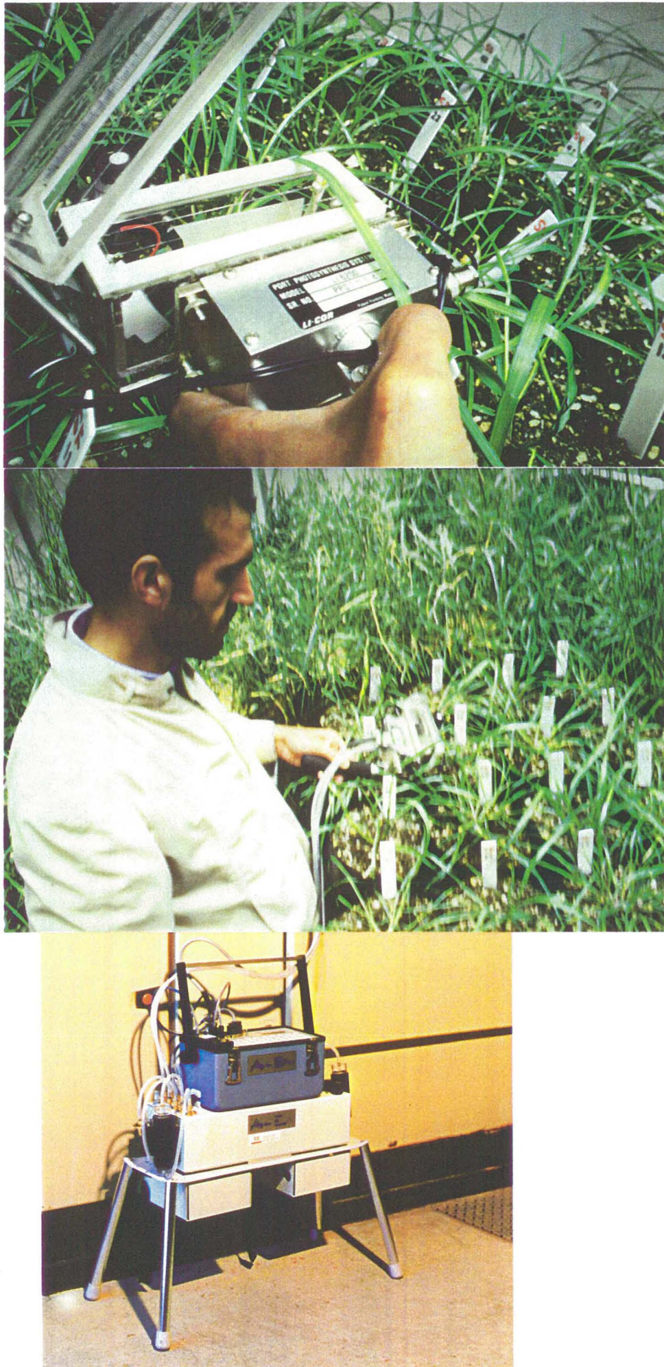
Plate 5.1: Measurement of leaf carbon exchange by Infra-red Gas Analyzer (Li-cor 6200)
